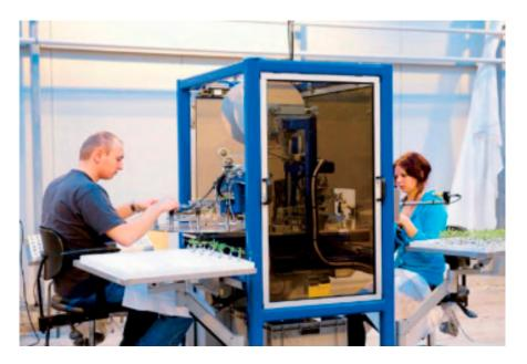
Figure 5. Graft1100 semi-automatic grafting robot developed by ISO Group.
