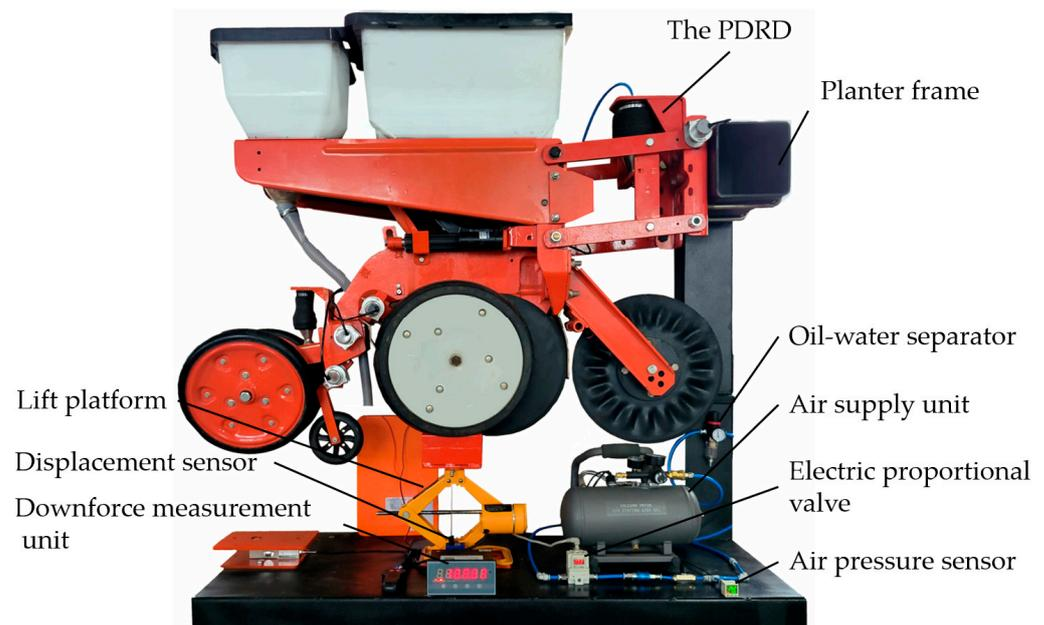
**Figure 7.** Seeding unit downforce test bench.
