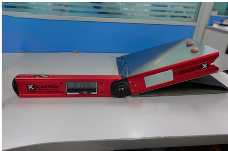
**Figure 7.** Static friction coefficient measuring device.
