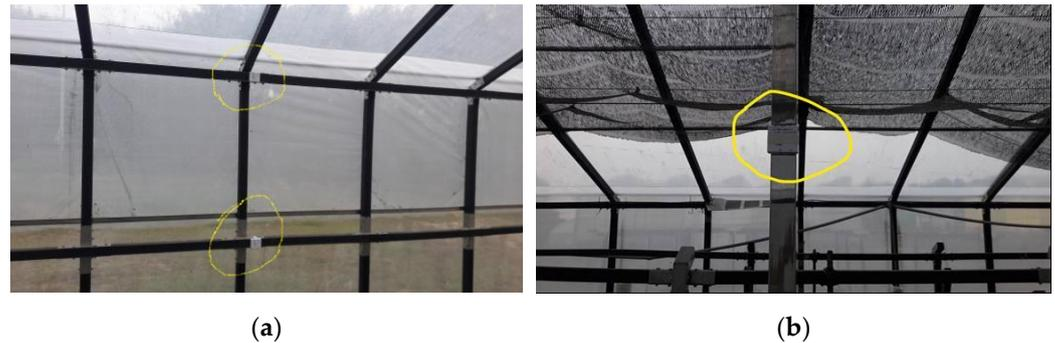
**Figure 9.** (a) Location of accelerometers on the gable frame; (b) location of accelerometer on the central stainless column.
