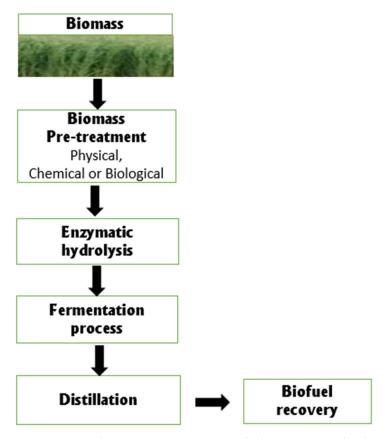
**Figure 1.** Schematic representation of the steps involved in biofuel production from lignocellulose biomass.
