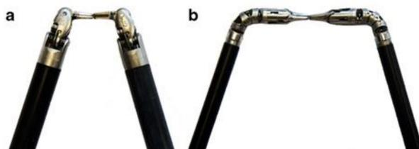
**Figure 6.** Comparison of the DaVinci 8 mm (a) and 5 mm diameter instruments (b). Due to their tentacle-like continuum tool shafts, the smaller diameter instruments need more operative space than the 8 mm instruments and are therefore not suitable in smaller cavities, such as infants. Figure taken from Marcus 2015 [62].
