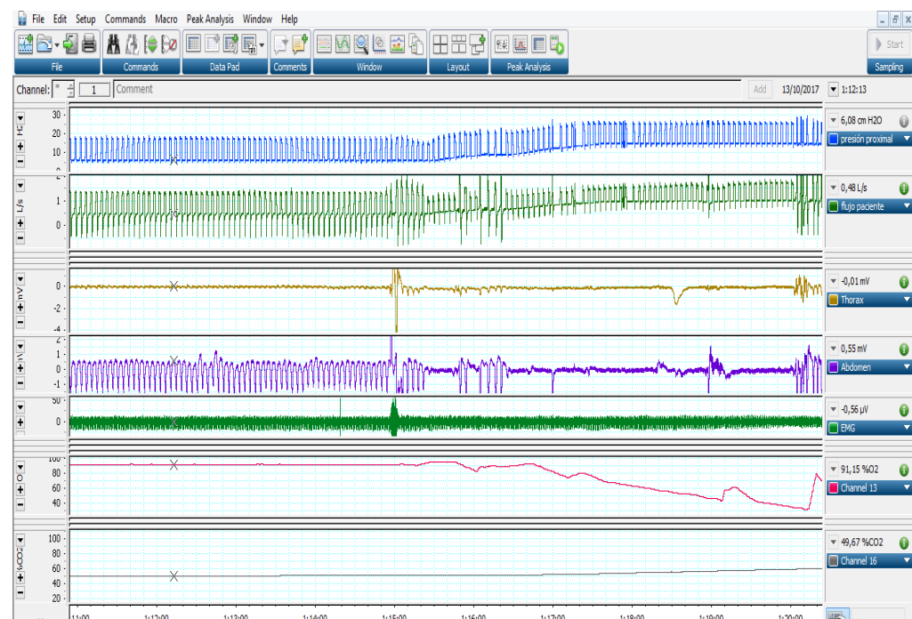
Figure 5. Example of inappropriate response of an automatic mode in a patient with UAO without effort (glottic closure). Observe the absence of movement in belts (Channels 3 and 4). In this case, the increase in pressure (Channel 1) was associated with a profound desaturation (Channel 6) and transcutaneous CO 2 increase (Channel 7).
