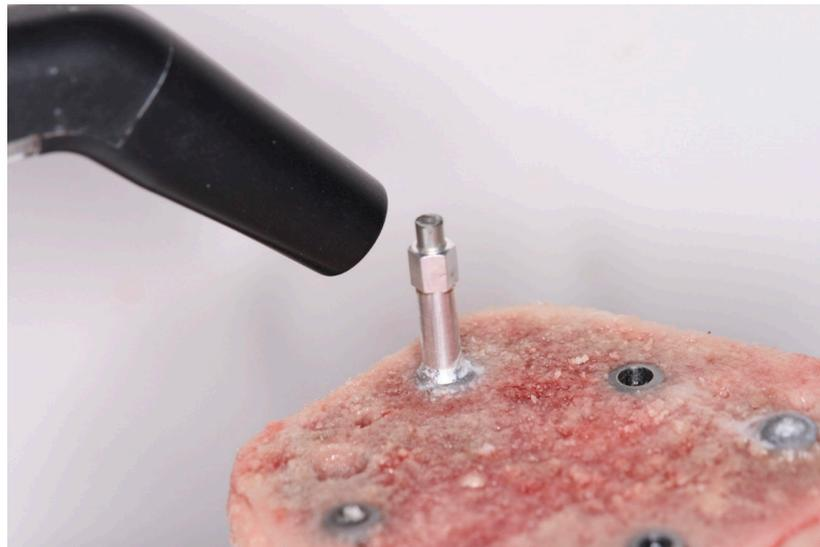
**Figure 4.** Implant stability quotient (ISQ) measurement of implant placed in the porcine tibia.
