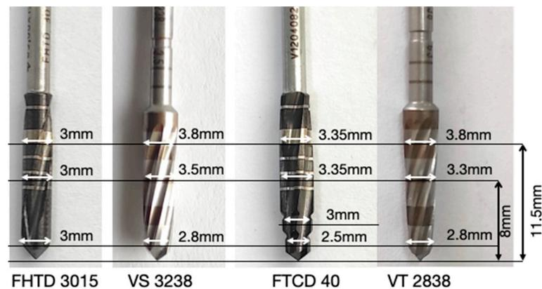
**Figure 2.** The configuration and dimensions of the final drill used for each group (1a, 1b, 2a and 2b).
