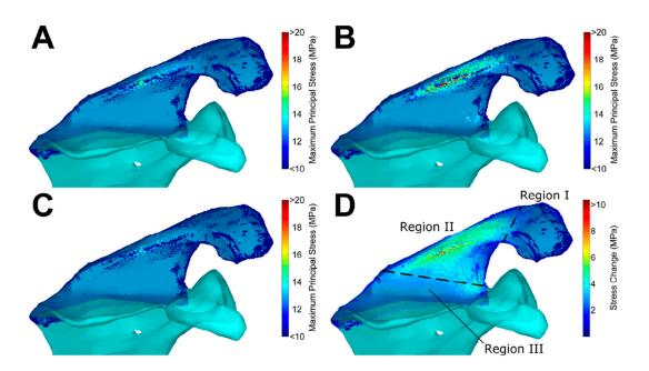
**Figure 3.** Finite element analysis on the influence of implant positioning in reverse total shoulder arthroplasty on acromial and scapular spine stresses by Wong et al. [47]. Reprinted with permission from ref. [47]. Copyright 2016 Elsevier. (A) Baseline implant configuration, (B) maximum stress configuration, (C) minimum stress configuration, and (D) stress increase from minimum to maximum stress configuration. Regions are as defined by Levy et al. [20].
