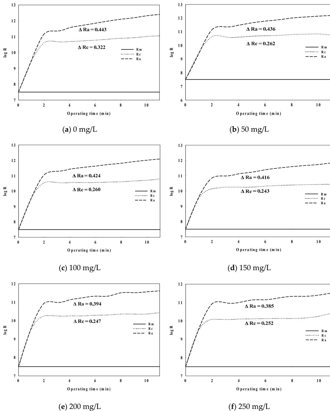
Figure 4. Behaviors of  $R_a$  and  $R_c$  with time.
