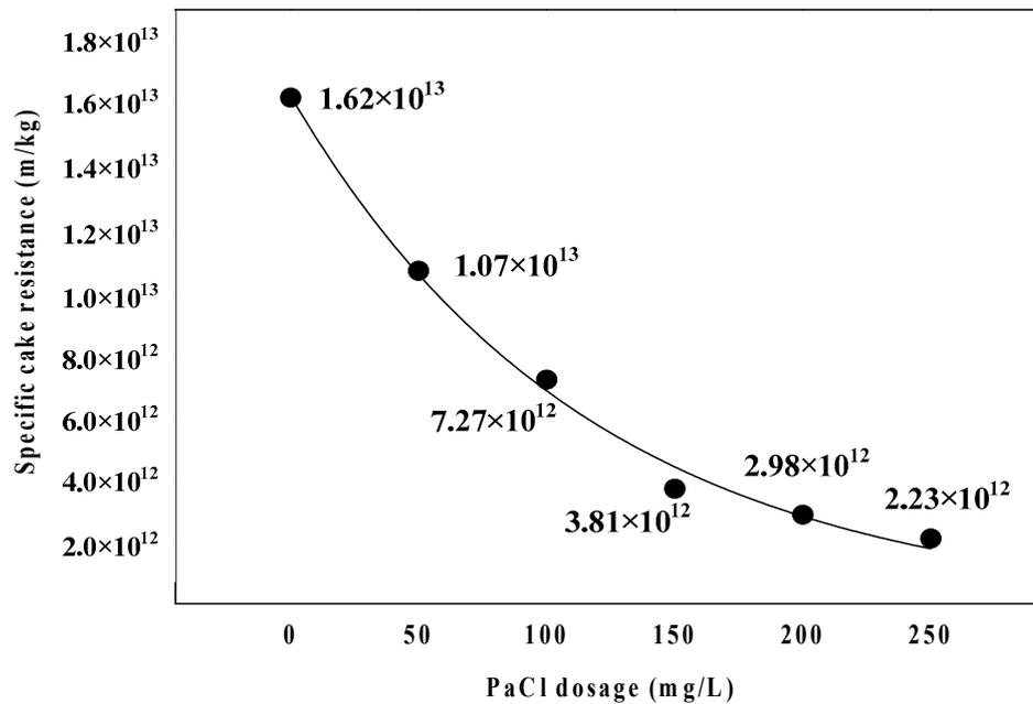
Figure 5. Comparison of cake specific cake resistance with coagulant dosage.
