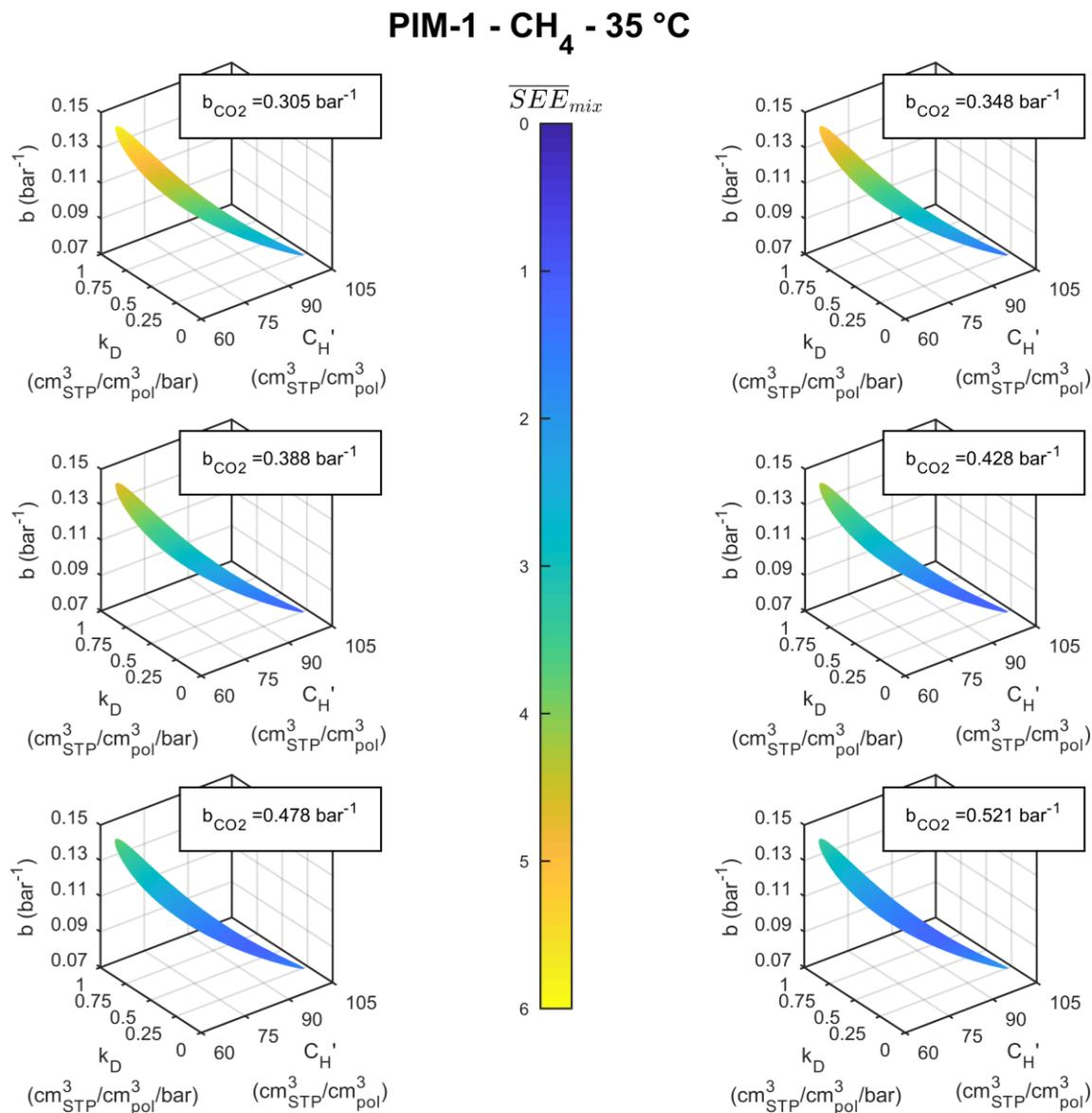
**Figure S6.** Isosurfaces the DMS model parameter space for CH<sub>4</sub> sorption in PIM-1 at 35 °C corresponding to  $SEE_{pure} < SEE_{max}$ , coloured according to the average  $SEE_{mix}$  obtained with different values within the confidence interval of  $b_{CO_2}$ .
