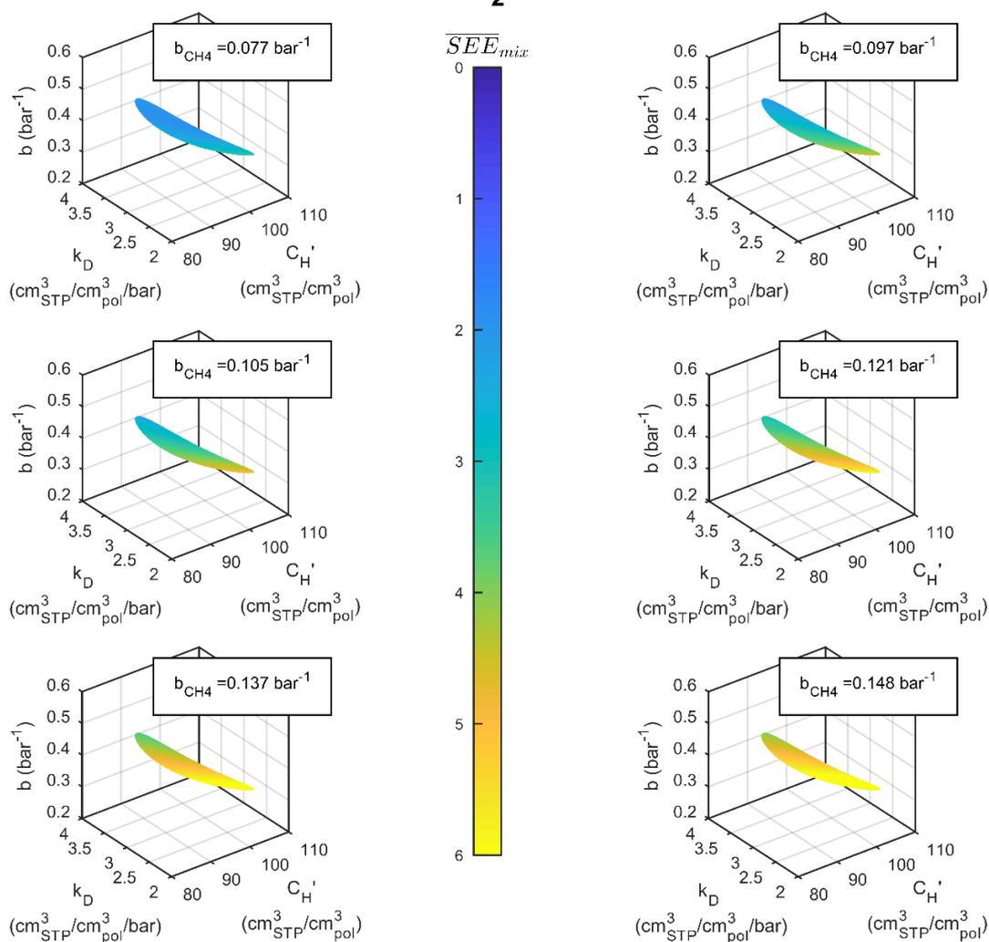
**Figure S11.** Isosurfaces the DMS model parameter space for CO<sub>2</sub> sorption in PIM-1 at 35 °C corresponding to  $SEE_{pure} < SEE_{max}$ , coloured according to the average  $SEE_{mix}$  obtained with different values within the confidence interval of  $b_{CH_4}$ .
