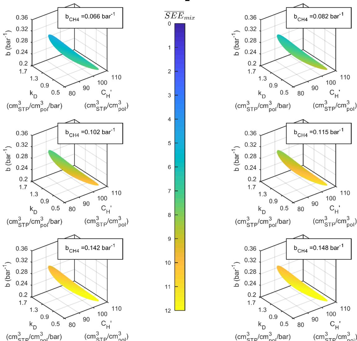
**Figure S20.** Isosurfaces in the DMS model parameter space for CO<sub>2</sub> sorption in TZ-PIM at 50 °C corresponding to  $SEE_{pure} < SEE_{max}$ , coloured according to the average  $SEE_{mix}$  obtained with different values within the confidence interval of  $b_{CH_4}$ .
