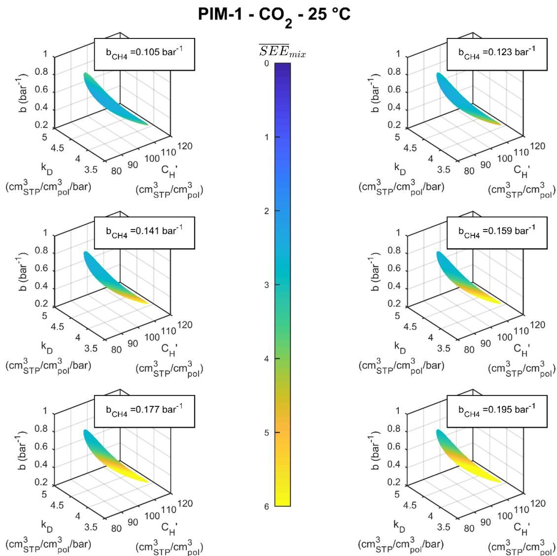
**Figure S10.** Isosurfaces the DMS model parameter space for  $CO_2$  sorption in PIM-1 at 25 °C corresponding to  $SEE_{pure} < SEE_{max}$ , coloured according to the average  $SEE_{mix}$  obtained with different values within the confidence interval of  $b_{CH_4}$ .
