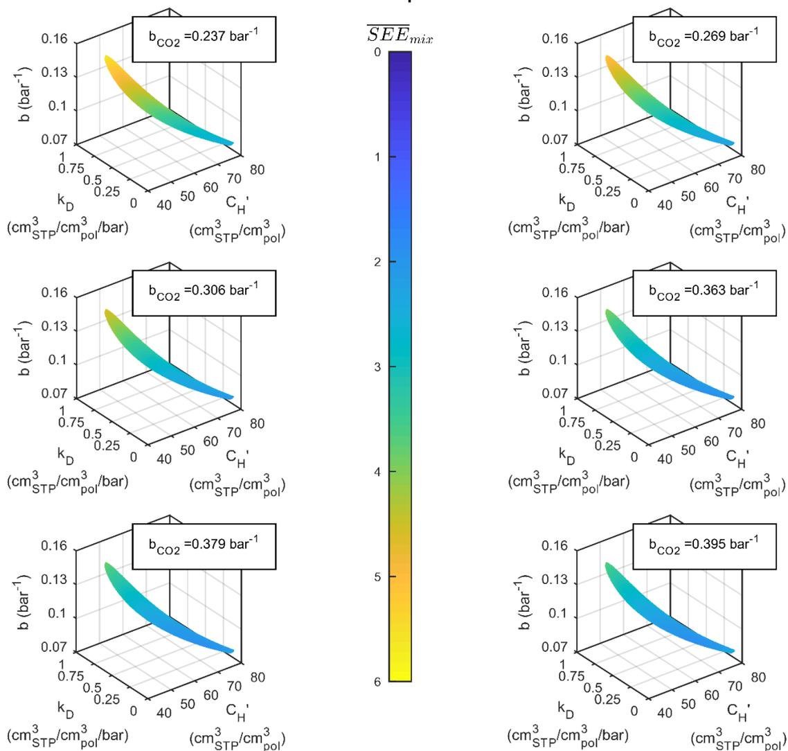
**Figure S7.** Isosurfaces the DMS model parameter space for CH<sub>4</sub> sorption in PIM-1 at 50 °C corresponding to  $SEE_{pure} < SEE_{max}$ , coloured according to the average  $\overline{SEE}_{mix}$  obtained with different values within the confidence interval of  $b_{CO_2}$ .
