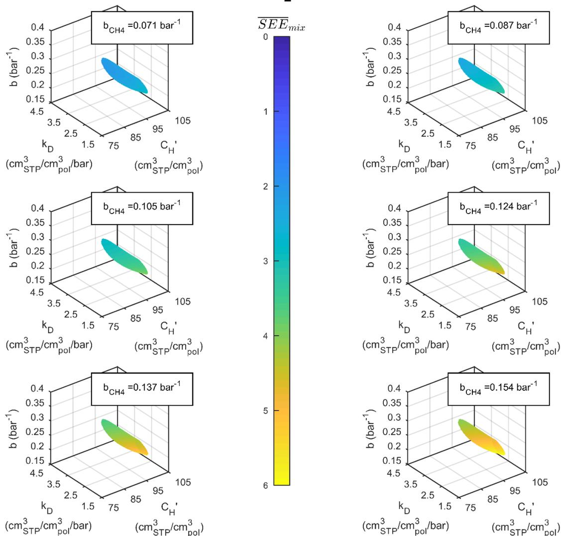
**Figure S12.** Isosurfaces in the DMS model parameter space for CO<sub>2</sub> sorption in PIM-1 at 50 °C corresponding to  $SEE_{pure} < SEE_{max}$ , coloured according to the average  $SEE_{mix}$  obtained with different values within the confidence interval of  $b_{CH_4}$ .
