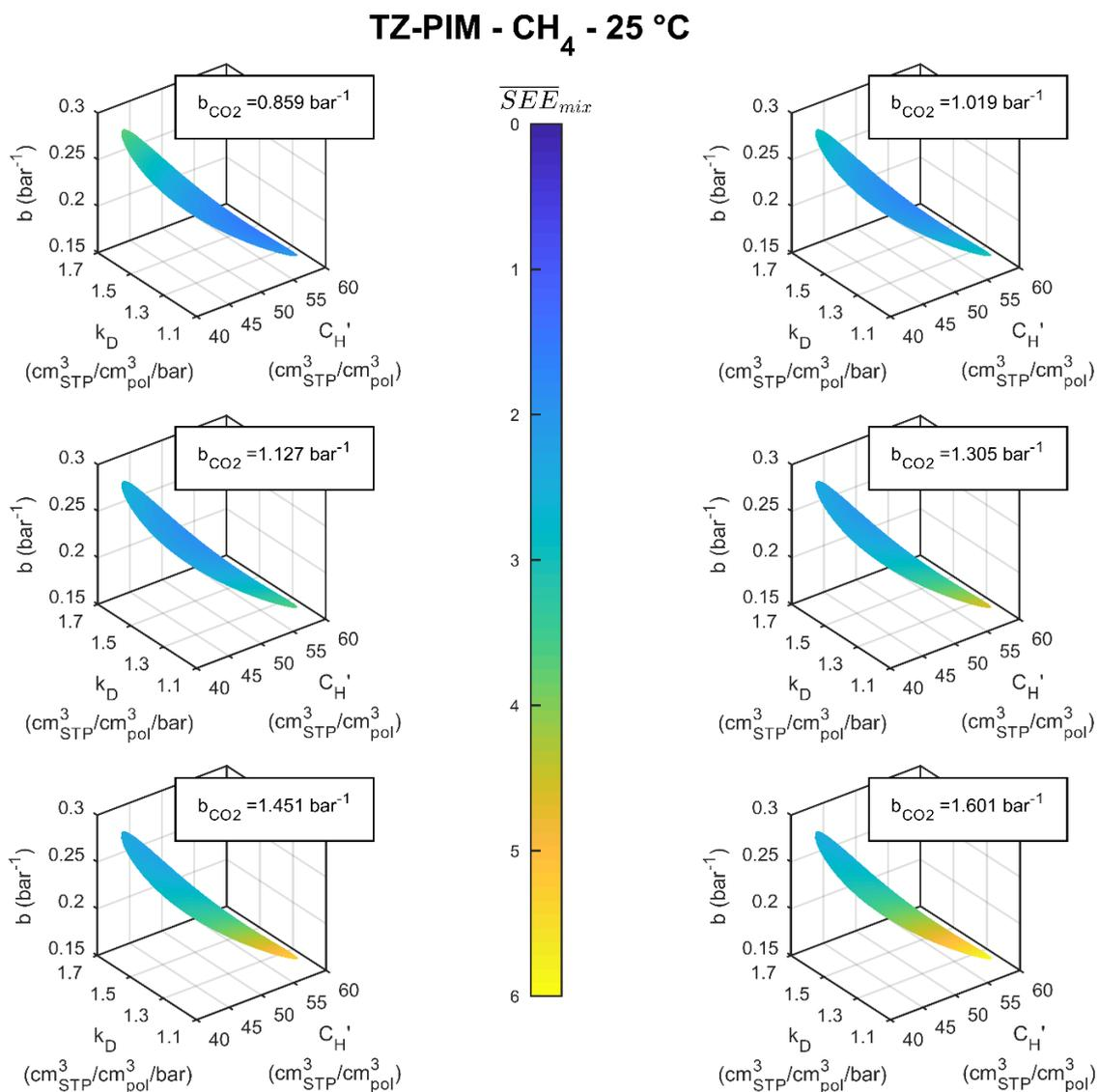
**Figure S15.** Isosurfaces in the DMS model parameter space for  $CH_4$  sorption in TZ-PIM at 25 °C corresponding to  $SEE_{pure} < SEE_{max}$ , coloured according to the average  $SEE_{mix}$  obtained with different values within the confidence interval of  $b_{CO_2}$ .
