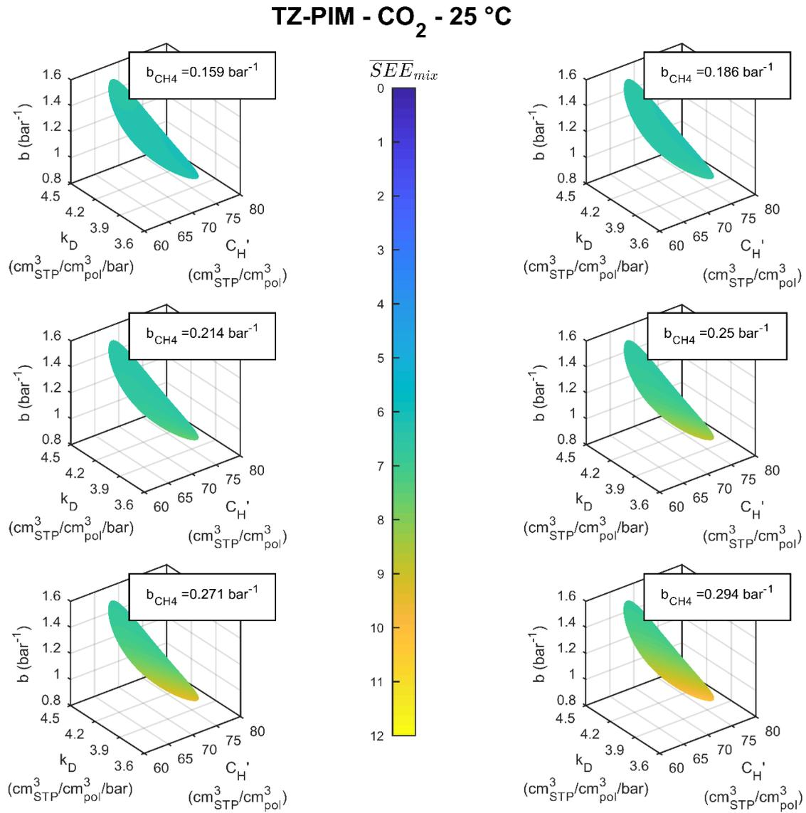
**Figure S18.** Isosurfaces in the DMS model parameter space for  $CO_2$  sorption in TZ-PIM at 25 °C corresponding to  $SEE_{pure} < SEE_{max}$ , coloured according to the average  $SEE_{mix}$  obtained with different values within the confidence interval of  $b_{CH_4}$ .
