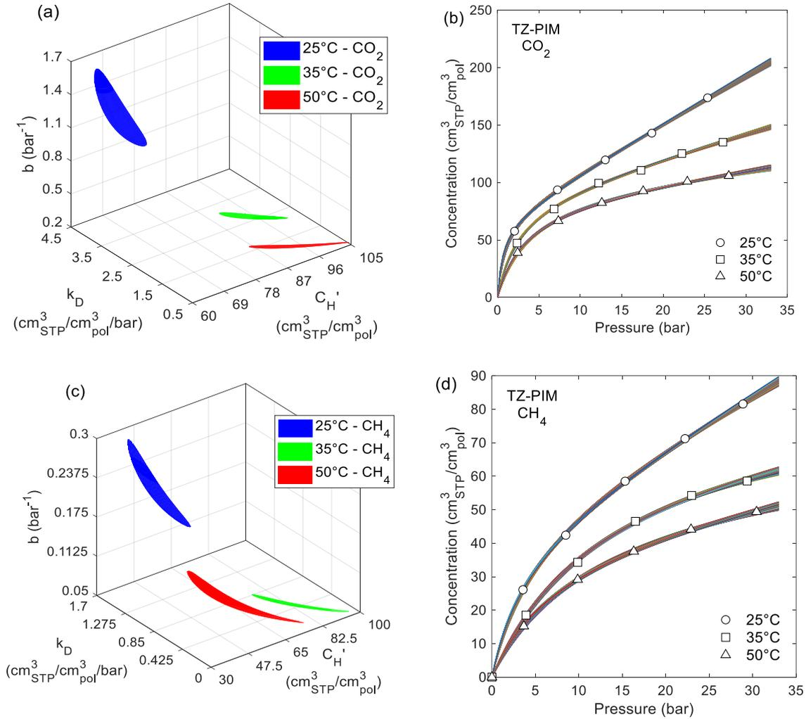
**Figure S13.** Surfaces enclosing the range where DMS parameter sets yield  $SEE < SEE_{max}$  in the prediction of (a) CO<sub>2</sub> and (c) CH<sub>4</sub> sorption in TZ-PIM at three different temperatures; (b) CO<sub>2</sub> and (d) CH<sub>4</sub> sorption isotherms in TZ-PIM calculated with all the parameter sets enclosed by the corresponding coloured region in the plot on the left.
