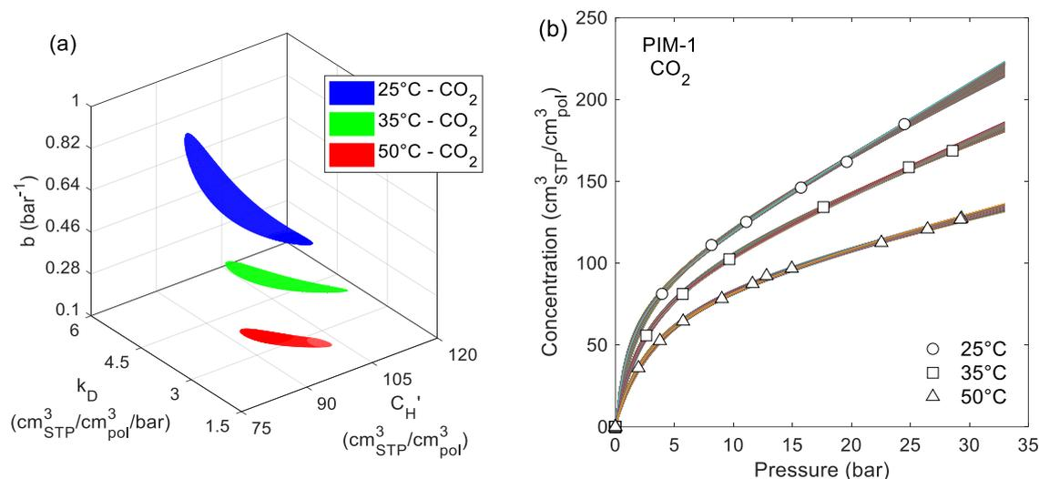
**Figure S8.** (a) Surfaces enclosing the range where DMS parameter sets yield  $SEE < SEE_{max}$  in the prediction of CO<sub>2</sub> sorption in PIM-1 at three different temperatures; (b) CO<sub>2</sub> sorption isotherms in PIM-1 at 25, 35 and 50 °C, calculated with all the parameter sets enclosed by the corresponding coloured regions in the plot on the left.
