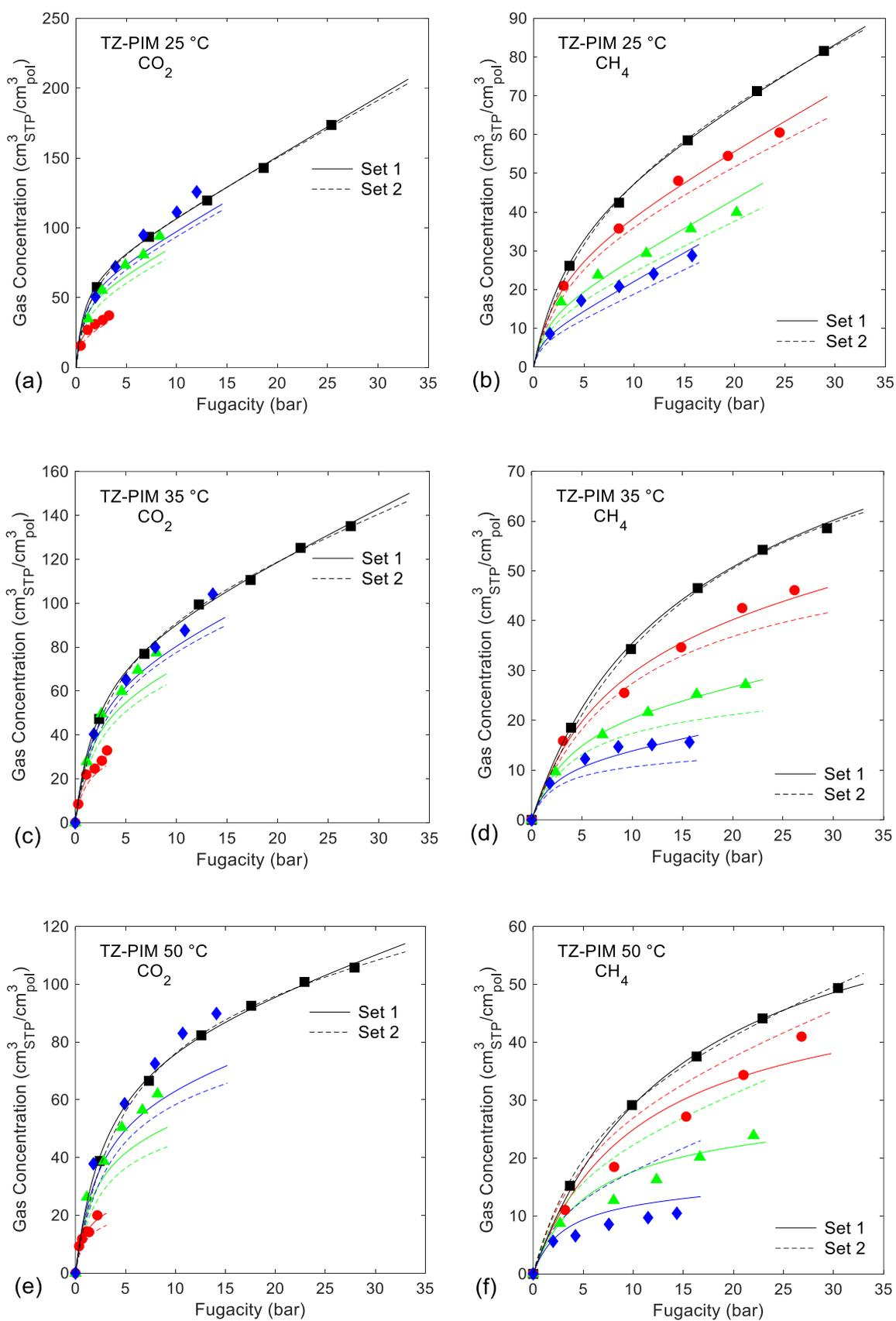
**Figure S14.** Dual Mode Sorption model mixed-gas predictions of  $\text{CO}_2$  and  $\text{CH}_4$  at 25 °C (a,b), 35 °C (c,d), 50 °C (e,f) in TZ-PIM, obtained with the two parameter sets reported in in Table S3. Solid lines are obtained with Set 1, dashed ones with Set 2.
