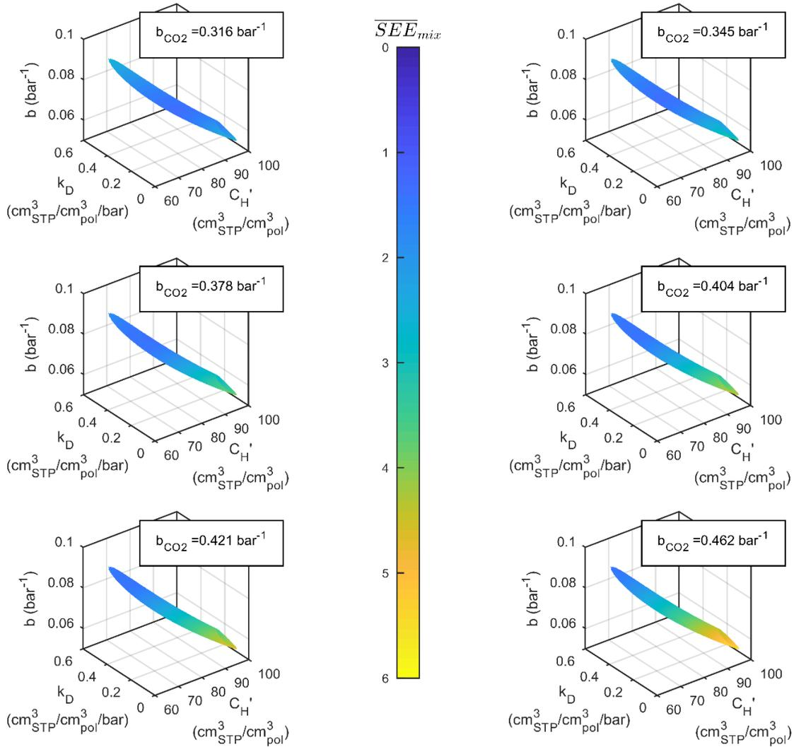
**Figure S16.** Isosurfaces in the DMS model parameter space for CH<sub>4</sub> sorption in TZ-PIM at 35 °C corresponding to  $SEE_{pure} < SEE_{max}$ , coloured according to the average  $SEE_{mix}$  obtained with different values within the confidence interval of  $b_{CO_2}$ .
