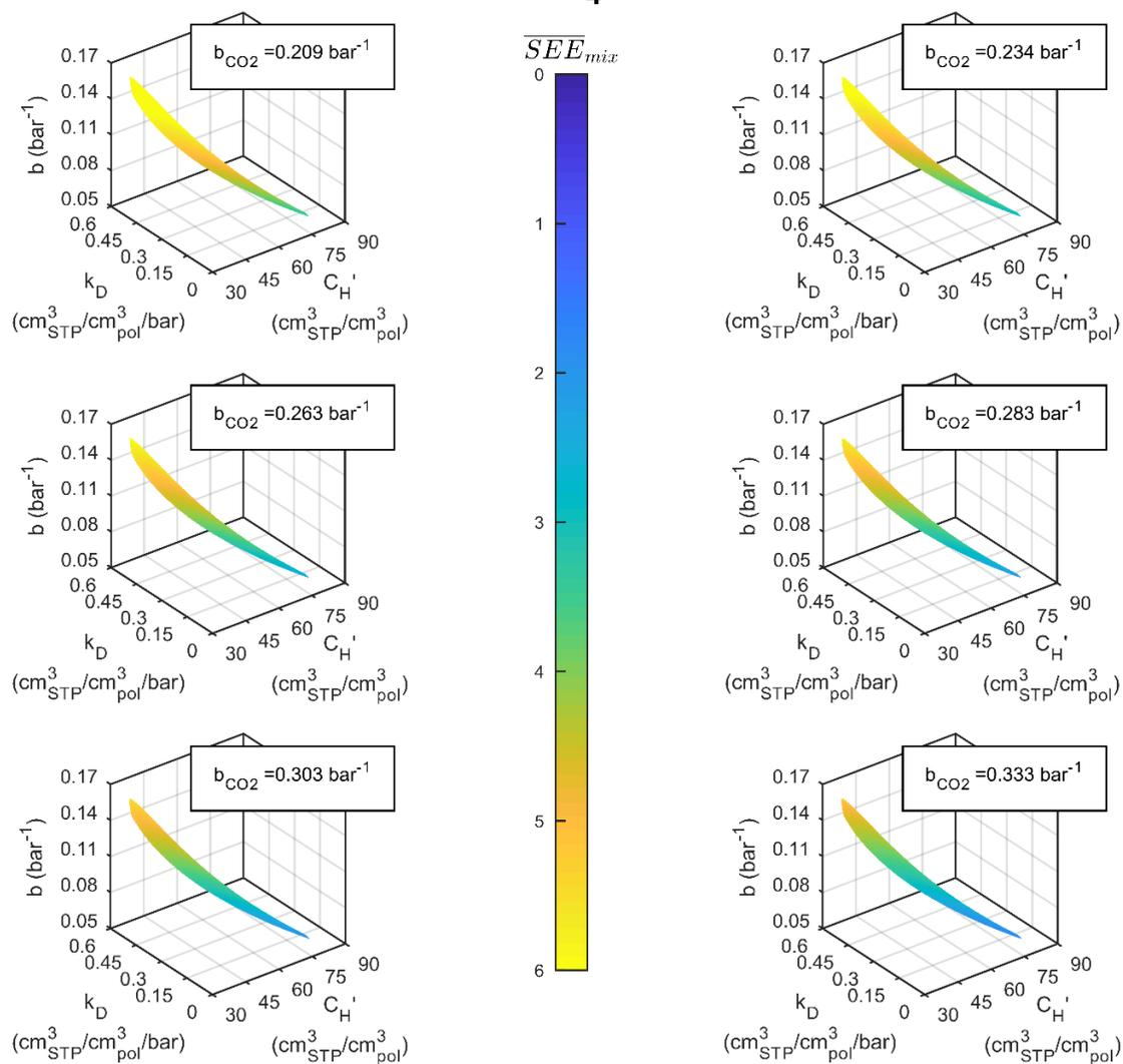
**Figure S17.** Isosurfaces in the DMS model parameter space for CH<sub>4</sub> sorption in TZ-PIM at 50 °C corresponding to  $SEE_{pure} < SEE_{max}$ , coloured according to the average  $SEE_{mix}$  obtained with different values within the confidence interval of  $b_{CO_2}$ .
