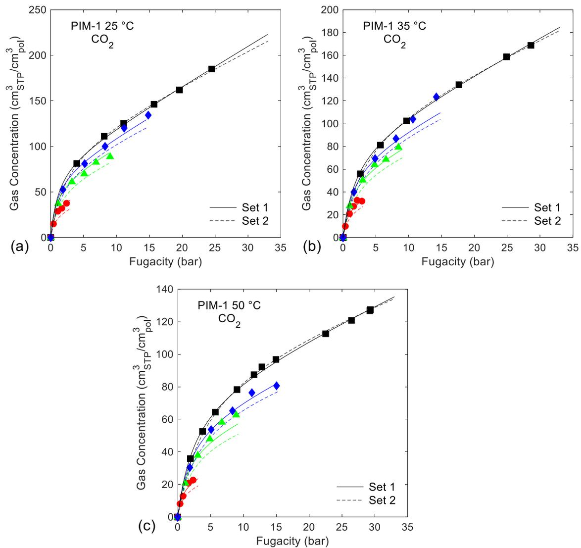
**Figure S9.** Dual Mode Sorption model mixed-gas predictions of CO<sub>2</sub> sorption in PIM-1 at 25 °C (a), 35 °C (b), 50 °C (c) obtained with the two parameter sets reported in Table S2.
