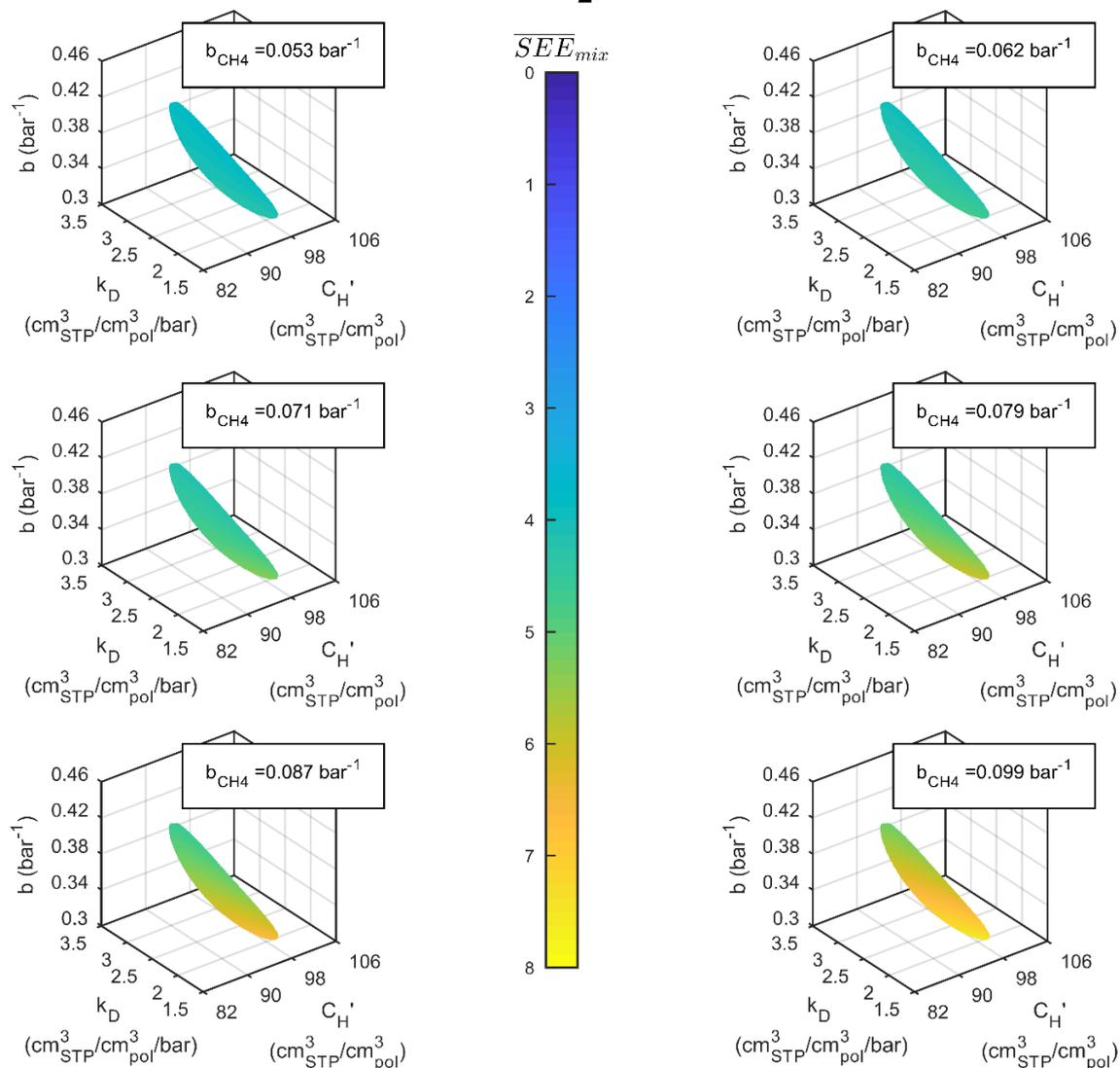
**Figure S19.** Isosurfaces in the DMS model parameter space for CO<sub>2</sub> sorption in TZ-PIM at 35 °C corresponding to  $SEE_{pure} < SEE_{max}$ , coloured according to the average  $SEE_{mix}$  obtained with different values within the confidence interval of  $b_{CH_4}$ .
