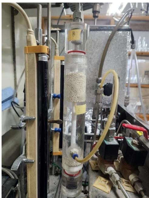
**Scheme 1.** Titanium dioxide-immobilized PES beads in the combined module of an alumina microfiltration membrane and PES beads.
