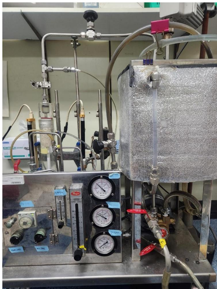
**Scheme 3.** The combined water treatment system of the tubular MF membrane and titanium dioxide-immobilized PES beads with intermittent air backwashing and UV radiation.
