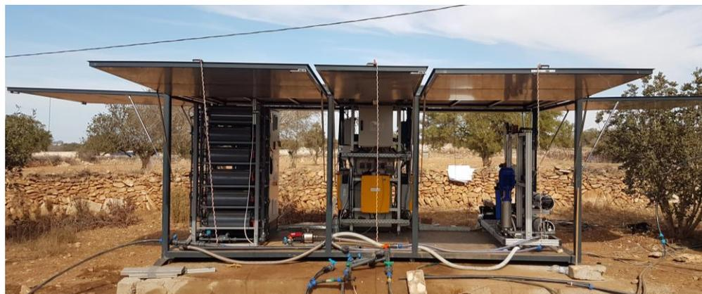
**Figure 1.** Smart Cube at pilot site of Essaouira: MCDI (left), power supply system (center), LPRO (right).
