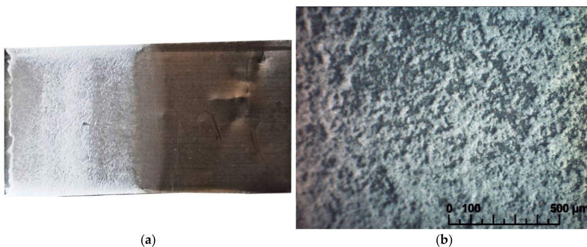
Figure 2. Surface of the dried LLZ coating obtained from a non-aqueous suspension of LLZ powder (10 g/L) during EPD on Ni-foil: (a) photo; (b) optical image.
