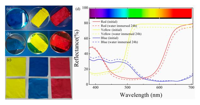
**Figure 8.** As-spun colored nanofibrous membranes (**a**) immersed in water; (**b**) after 24 h; (**c**) comparing membranes before and after immersion in water; and (**d**) UV-Vis diffuse reflectance spectroscopy of these membranes. From [173], copyright (2016), originally published under a CC-BY license.
