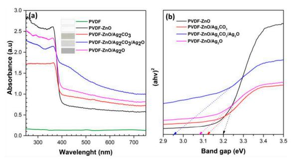
**Figure 2.** (a) Absorbance spectra, (b) band gap determination by drawing the line at  $(\alpha h\nu)^2$  of the electrospun nanofibers. For polyvinylidene fluoride (PVDF), no band gap could be calculated since the absorbance was too low. From [55], copyright (2019), originally published under a CC-BY license.
