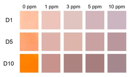
**Figure 7.** Color changes of each nanofiber sensor after exposure to various NH<sub>3</sub> concentrations (1, 3, 5, and 10 ppm). Nanofibrous sensors D1, D5, and D10 contain 1%, 5%, and 10% of the dye, respectively. From [166], copyright (2020), originally published under a CC-BY license.
