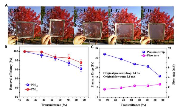
**Figure 3.** (**A**) Photographs of PDMS/PMMA-chitosan transparent air filters at different transparencies; (**B**) PM<sub>2.5</sub> and PM<sub>10</sub> removal efficiency; and (**C**) pressure drop and flow rate of transparent filters at different transmittances. From [74], copyright (2019), originally published under a CC-BY license.
