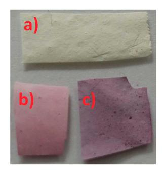
**Figure 6.** Photograph of differently treated electrospun nanofiber mats: (**a**) pure PAN-TiO<sub>2</sub>; (**b**) PAN after dip-coating in anthocyanin dye solution and drying; (**c**) PAN-TiO<sub>2</sub> after dyeing, showing a bathochromic shift. From [158], copyright (2022), originally published under a CC-BY-SA license.
