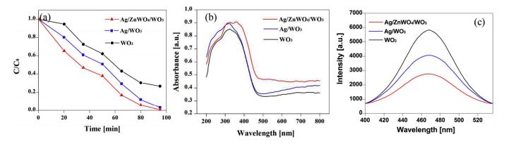
**Figure 1.** (a) Photocatalytic decomposition of methylene blue with WO<sub>3</sub>, Ag/WO<sub>3</sub>, and Ag/ZnWO<sub>4</sub>/WO<sub>3</sub> composites nanofibers, (b) UV/Vis diffuse reflectance spectra, and (c) photoluminescence spectra of as-prepared samples. From [50], copyright (2019), with permission from Elsevier.
