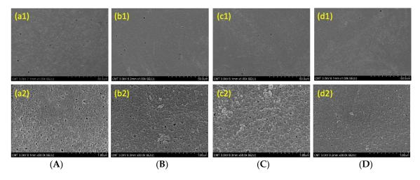
**Figure 1.** The outer surface SEM images of TA-FeIII/PAN membranes with different treatment time. **(A)** 0 min, **(B)** 1 min, **(C)** 2 min, **(D)** 3 min. Magnification (a1–d1) 1 K, (a2–d2) 50 K.
