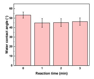
Figure 3. Water contact angle of the membranes, coated at different reaction times, of TA and FeIII.
