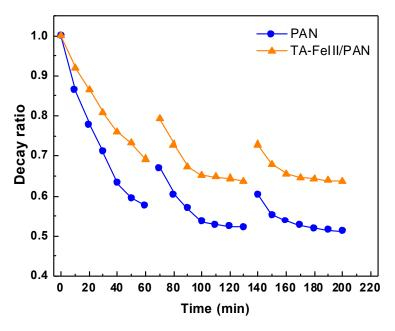
**Figure 6.** Reusability test of PAN and TA-FeIII membranes. Feed:  $H_2O/diesel$  (99/1) emulsion at 1 bar.
