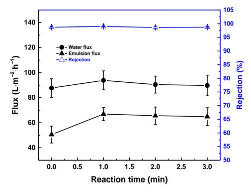
Figure 4. Effect of reaction time between TA and FeIII. Feed: H<sub>2</sub>O/diesel (99/1) emulsion at 1 bar.
