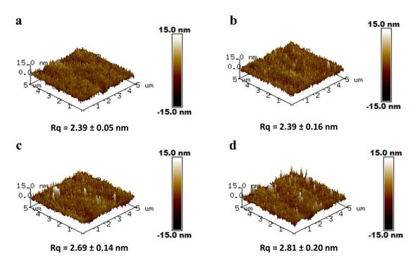
**Figure 2.** Three-dimensional AFM images of the membranes coated at different reaction times of TA and FeIII: (a) PAN; (b) 1 min; (c) 2 min; (d) 3 min; Lateral scale =  $5 \mu$ m. Vertical scale = -15 to 15 nm.
