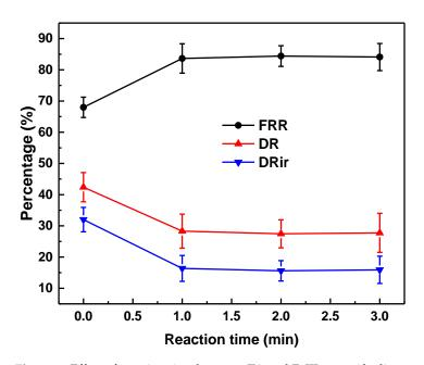
**Figure 5.** Effect of reaction time between TA and FeIII on antifouling performance. Feed:  $H_2O/diesel$  (99/1) emulsion at 1 bar.
