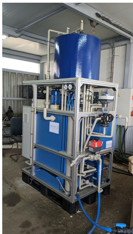
**Figure 2.** Commercial MD system used in the experimental campaign.
