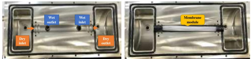
Figure 1. A configuration of a hollow-fiber membrane humidifier.
