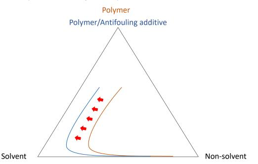
**Figure 4.** Schematic effect of the antifouling additive on the position of the demixing gap. Red arrows highlight the shift of the binodal line towards the solvent/polymer axis.
