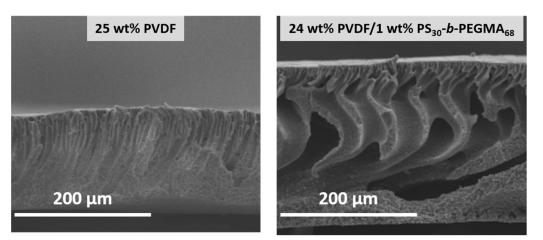
**Figure 5.** Influence of the addition of 1 wt%  $PS_{30}$ -*b*-PEGMA<sub>68</sub> copolymer to a casting solution containing PVDF (NMP as solvent) on the cross-sectional morphology of LIPS membranes ( $T_{dissolution}$ : 40 °C; Solvent content fixed: 75 wt%; non-solvent: DI water; casting thickness: 300 µm). Left image partially reproduced with permission from [357]. Copyright 2014 Elsevier.
