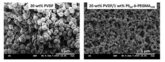
**Figure 6.** Influence of the addition of 1 wt% PS<sub>60</sub>-*b*-PEGMA<sub>108</sub> copolymer to a casting solution containing 20 wt% PVDF (NMP as solvent) on the surface morphology of VIPS membranes ( $T_{dissolution}$ : 32 °C; RH: 70%;  $T_{chamber}$ : 25 °C;  $t_{exposure}$ : 20 min; casting thickness: 300 µm).
