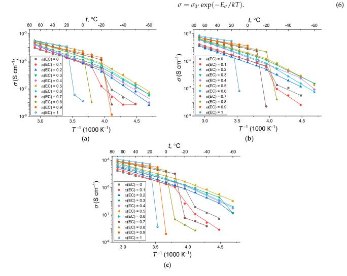
**Figure 5.** Temperature dependence of ionic conductivity of the Na-Nafion membranes, swollen at (a)  $40 \degree C$ , (b)  $60 \degree C$ , (c)  $80 \degree C$ .
