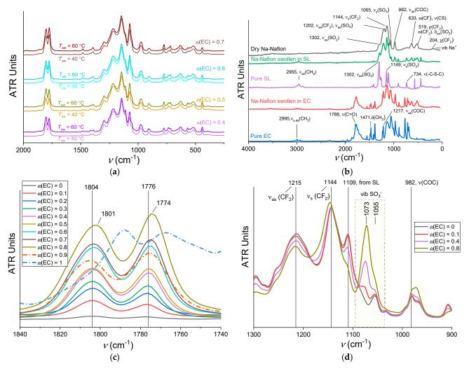
**Figure 9.** (a) The survey FTIR ATR spectra of Na-Nafion membranes swollen at 40 and 60 °C. (b) The survey FTIR ATR spectra of Nafion membrane dried over  $P_2O_5$ , initial solvents EC and SL and swollen Na-Nafion membranes. (c) Contours of the analytical band  $\nu$ (C=O) of EC in the FTIR ATR spectra of swollen Na-Nafion. (d) Contours of the analytical band  $\nu$ (SO) of the Na-Nafion (shaded area) in the FTIR ATR spectra of plasticized Na-Nafion.
