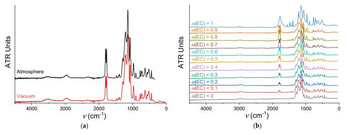
**Figure 8.** The survey FTIR ATR spectra of swollen Na-Nafion membranes: (**a**) recorded at various conditions ( $\omega(\text{EC}) = 0.5$ ,  $T_{sw} = 40 \text{ °C}$ ); (**b**) with various  $\omega(\text{EC})$ ; swollen at 40 °C and swollen at 40 and 60 °C.
