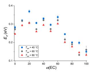
**Figure 6.** Dependence of the activation energy of conductivity on the EC content in mixture EC–SL above the kink temperature.
