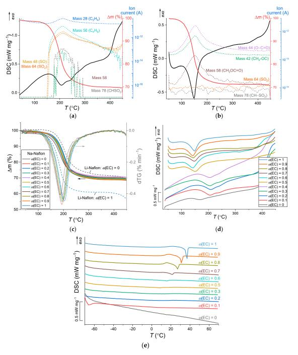
**Figure 4.** STA and ion current flow curves of the membrane swollen at 40 °C in (**a**) pure SL and (**b**) pure EC; (**c**) TGA curves (solid lines) and the first derivatives of the TGA curves (dotted lines) (for comparison, the TGA curves for the Li-Nafion are shown by dashed lines) and (**d**) DSC curves of the Na-Nafion membranes; (**e**) DSC curves in the low temperature region during heating.
