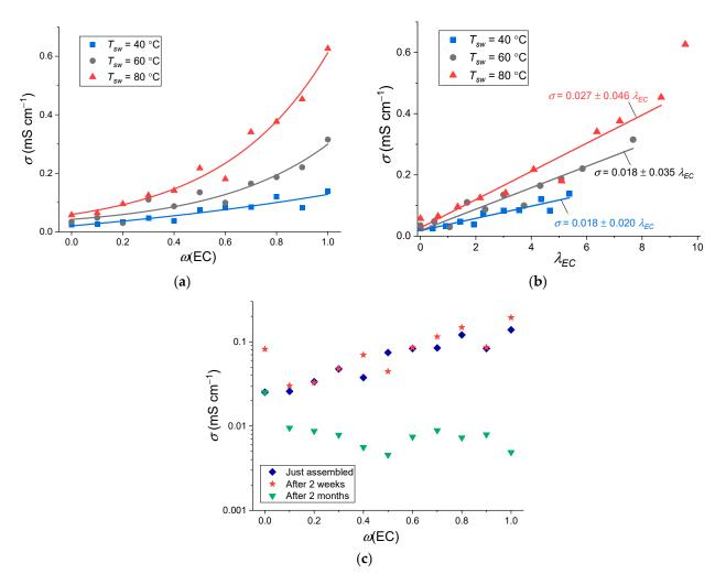
**Figure 7.** Ionic conductivity of the membranes at 30 °C for Na-Nafion membranes swollen at various temperatures as a function of (a)  $\omega(\text{EC})$  and (b)  $\lambda_{EC}$ ; (c) ionic conductivity of the membranes at 30 °C at various measurement times ( $T_{sw} = 40$  °C).
