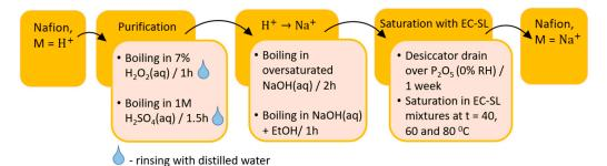
Figure 2. Scheme for obtaining the sodium form of Nafion membranes.
