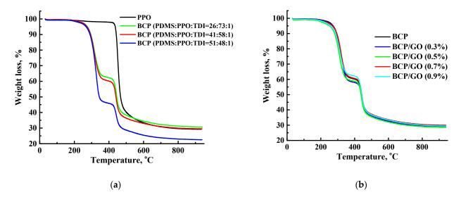
Figure 11. Thermogravimetric (TG) curves for the (a) PPO and BCP and (b) BCP and BCP/GO membranes.
