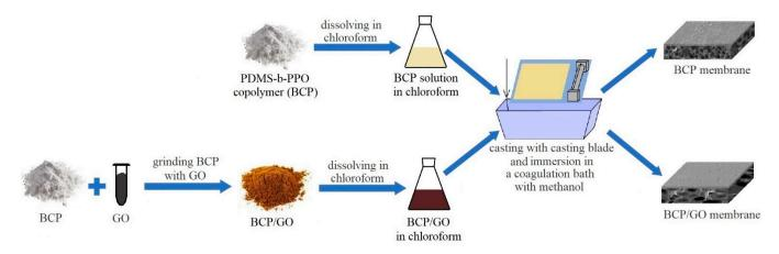
Figure 2. Preparation scheme of the BCP-based membranes.
