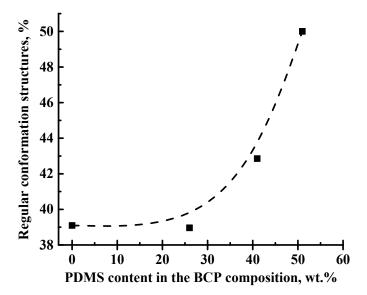
**Figure 8.** The dependence of regular conformation structure proportion on the PDMS content in the BCP composition.
