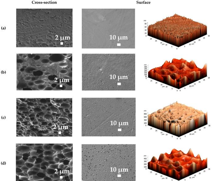
Figure 9. Cross-sectional and surface SEM micrographs and AFM images of the (a) PPO and BCP (b) PDMS:PPO:TDI = 26:73:1, (c) PDMS:PPO:TDI = 41:58:1 and (d) PDMS:PPO:TDI = 51:48:1 membranes.
