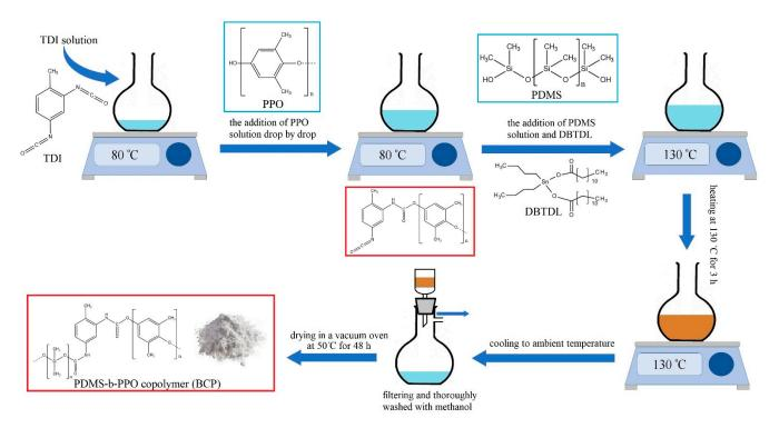
Figure 1. The scheme of a block copolymer (BCP) preparation.
