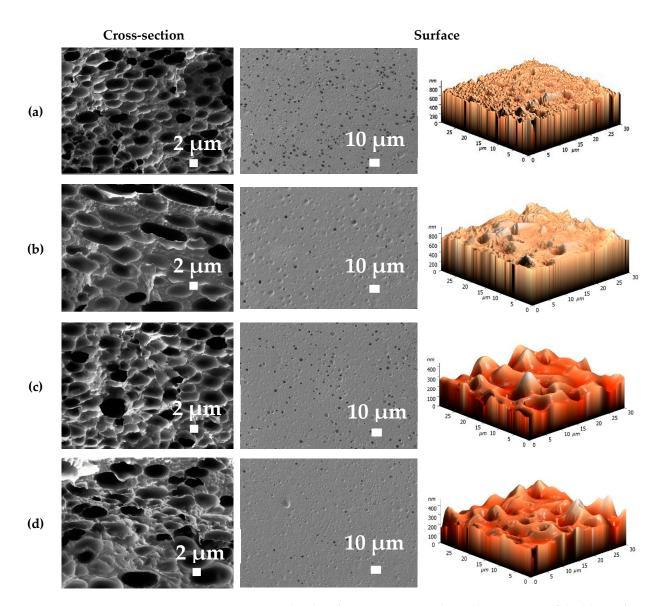
**Figure 10.** Cross-sectional and surface SEM micrographs and AFM images of the (**a**) BCP/GO (0.3%), (**b**) BCP/GO (0.5%), (**c**) BCP/GO (0.7%) and (**d**) BCP/GO (0.9%) membranes.
