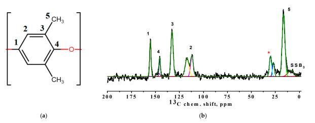
**Figure 7.** (a) Schematic representation of a PPO monomer with numbered nonequivalent carbon atoms (1, 2, 3, 4, and 5) and (b)  $^{13}$ C NMR spectrum of the BCP membrane. Asterisk refers to the group of peaks at about 30 ppm corresponding to the methyl groups of PDMS.
