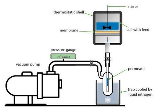
Figure 3. Schematic of pervaporation setup.
