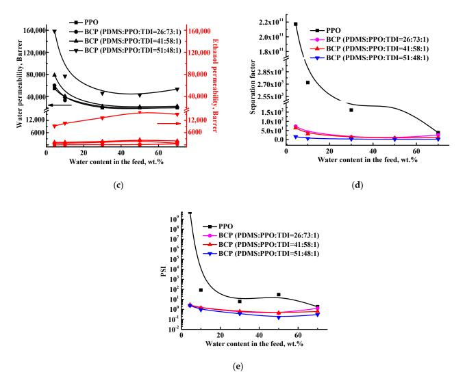
**Figure 4.** The dependence of (a) permeation flux, (b) water content in the permeate, (c) component permeability, (d) separation factor and (e) PSI on water content in the feed for the PPO and BCP-based membranes in pervaporation dehydration of ethanol (4.4-70 wt.% water) at 22 °C.
