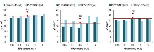
Figure 5. The specific surface free energy (overall (left), polar (center), and dispersive (right)).
