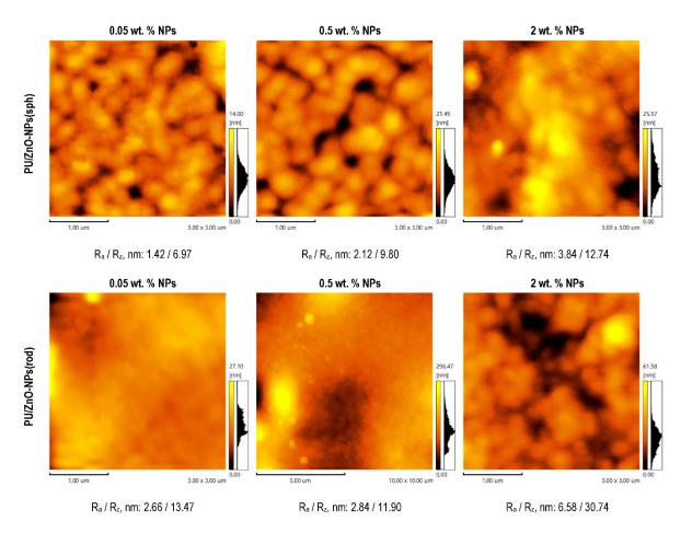
Figure 4. The AFM data of the membranes based on the various PU solutions with ZnO-NPs.
