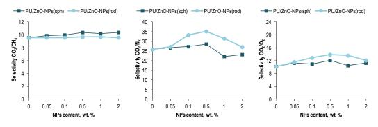
Figure 7. The selectivity of the polymeric membranes based on the PU/ZnO-NPs.
