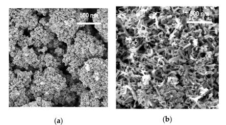
**Figure 2.** The SEM images of the spherical (a) and rod-shaped (b) ZnO-NPs obtained by the PECVD method.
