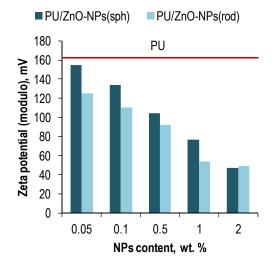
Figure 3. The zeta potential of the polymer solutions based on PU/ZnO-NPs in THF.
