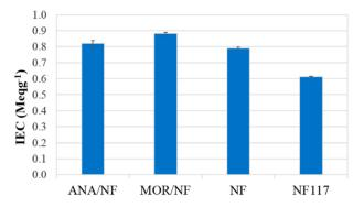
**Figure 4.** IEC of zeolite/Nafion membranes compared with recast Nafion and Nafion 117 membrane. Reprinted with permission from Ref. [83]. Copyright 2017 Elsevier.
