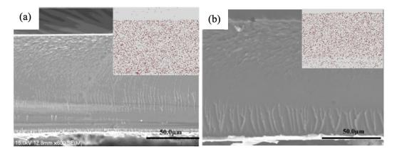
**Figure 5.** SEM images for  $NH_4 - X$  zeolite/Nafion composite membrane with 5 wt% of: (a) nano and; (b) submicron  $NH_4 - X$  zeolite. Reprinted with permission from Ref. [85]. Copyright 2015 Elsevier.
