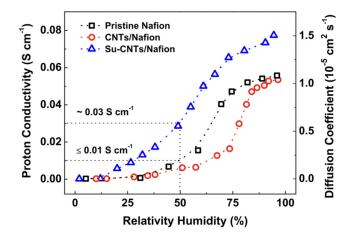
**Figure 11.** Proton conductivity and proton diffusion coefficient of membranes as a function of relative humidity. Reprinted with permission from Ref. [119]. Copyright 2018 American Chemical Society.
