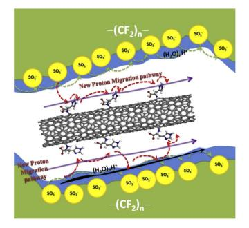
**Figure 12.** Interaction between nitrogen groups of imidazole–functionalized CNT and H<sup>+</sup>. Reprinted with permission from Ref. [108]. Copyright 2013 Elsevier.
