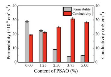
**Figure 7.** Methanol permeability and conductivity of pristine Nafion and PSAO–based Nafion composite membranes. Reprinted with permission from Ref. [101]. Copyright 2018 Elsevier.
