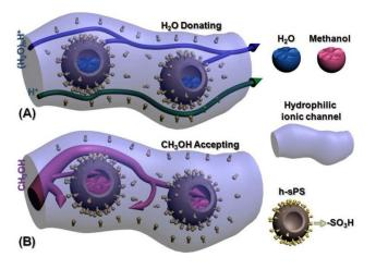
**Figure 6.** Schematic illustrations of "H<sub>2</sub>O donating/methanol accepting" mechanism: (**a**) releasing of free water and; (**b**) blocking of methanol. Reprinted with permission from Ref. [91]. Copyright 2015 Royal Society of Chemistry.
