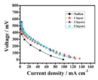
**Figure 2.** MEA performance of Nafion impregnated multilayer PVDF fibrous membranes with 10 M methanol. Reprinted with permission from Ref. [54]. Copyright 2019 Wiley-VCH.
