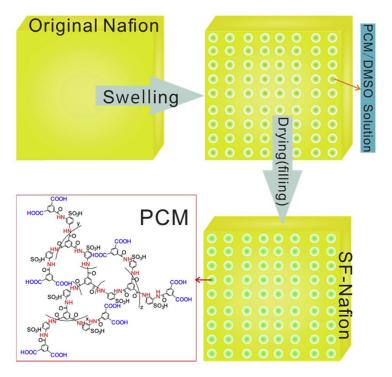
**Figure 3.** Schematic illustration of in situ swelling–filling Nafion modification strategy. Reprinted with permission from Ref. [65]. Copyright 2016 Elsevier.
