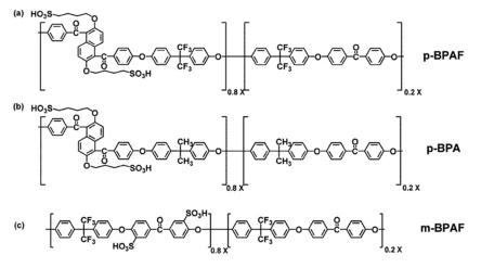
**Figure 1.** Chemical structures of three types of SPAEK blending modifiers: (**a**) p–BPAF; (**b**) p–BPA; (**c**) m–BPAF. Reprinted with permission from Ref. [48]. Copyright 2018 Elsevier.
