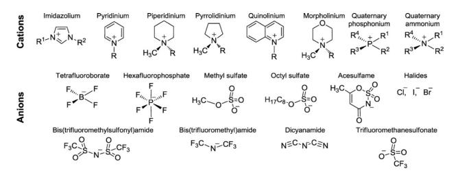
**Figure 9.** Structure of commonly used cations and anions in ionic liquid. Reprinted with permission from Ref. [111]. Copyright 2017 American Chemical Society (United States).
