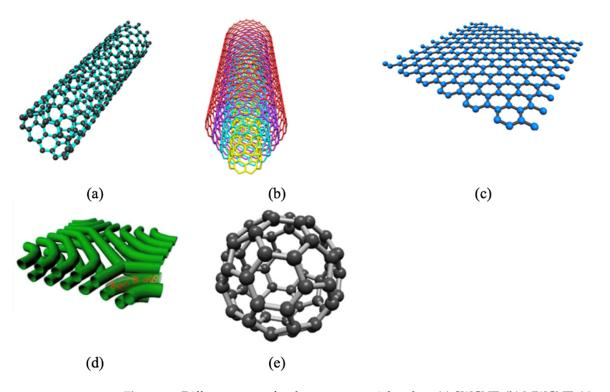
**Figure 10.** Different types of carbon nanomaterial such as (**a**) SWCNT; (**b**) MWCNT; (**c**) graphene; (**d**) mesoporous carbon; (**e**) fullerene. Reprinted with permission from Ref. [114]. 2013, Elsevier; Reprinted with permission from Ref. [115]. Copyright 2013 American Chemical Society (United States).
