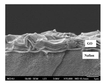
**Figure 13.** SEM image of the GO–laminated Nafion membrane. Reprinted with permission from Ref. [122]. Copyright 2013 Elsevier.
