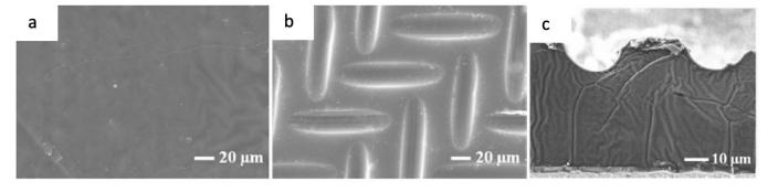
**Figure 15.** SEM image of (**a**) unmodified; (**b**) and (**c**) hot–mold–modified of Nafion membrane. Reprinted with permission from Ref. [133]. Copyright 2017 Elsevier.
