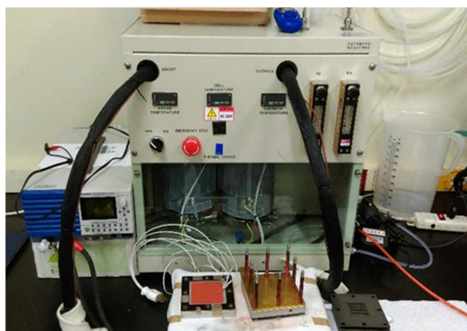
Figure 4. A machine for measuring fuel cells.
