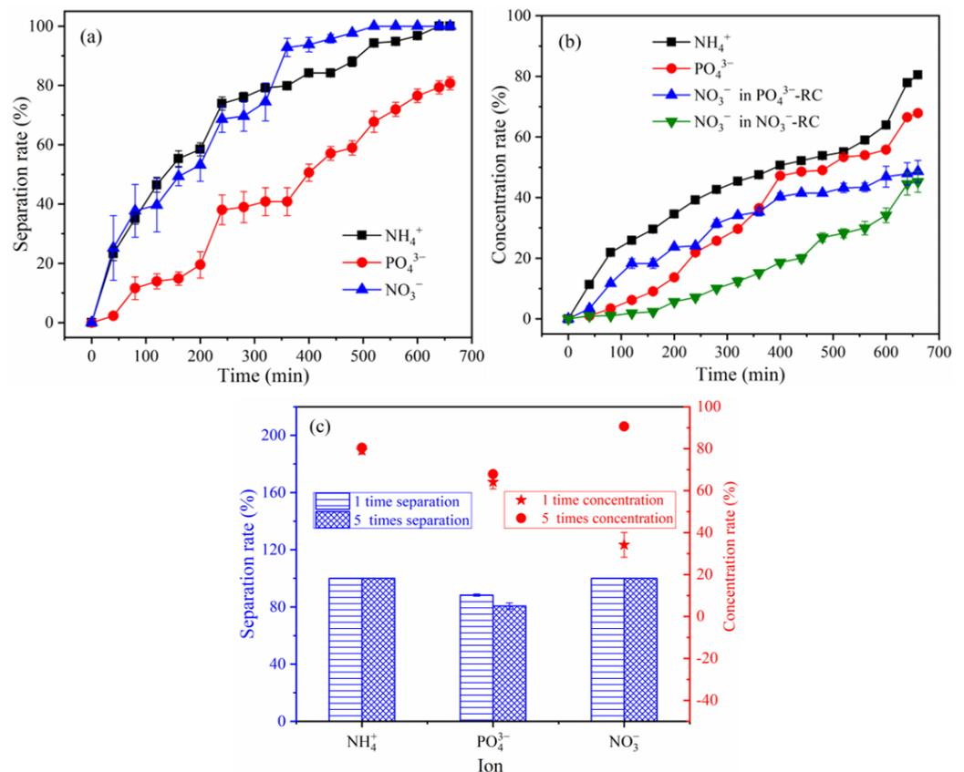
**Figure 7.** (a) separation and (b) concentration of  $\text{NH}_4^+$ ,  $\text{PO}_4^{3-}$  and  $\text{NO}_3^-$  with the volume ratio of  $V_{\text{WWC}}/V_{\text{AWC}}$ ,  $V_{\text{WWC}}/V_{\text{PC}}$ , and  $V_{\text{WWC}}/V_{\text{NAC}}$  was 5:1 and (c) the comparison with volume ratio of  $V_{\text{WWC}}/V_{\text{AWC}}$ ,  $V_{\text{WWC}}/V_{\text{PC}}$ , and  $V_{\text{WWC}}/V_{\text{NAC}}$  was 1:1.
