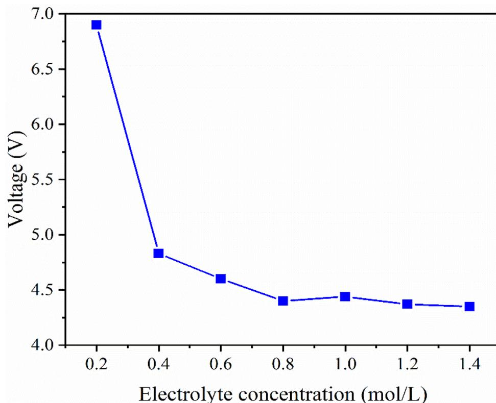
**Figure 2.** Cell voltage variation of cell voltage with  $\text{Na}_2\text{SO}_4$  concentration.
