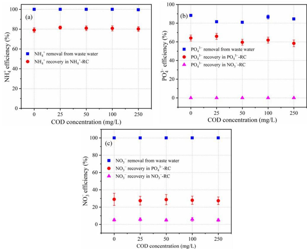
**Figure 6.** Effect of COD concentration on the separation and concentration of (a)  $\text{NH}_4^+$ , (b)  $\text{PO}_4^{3-}$  and (c)  $\text{NO}_3^-$ .
