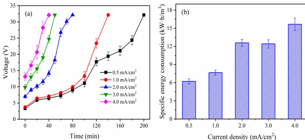
**Figure 4.** (a) Voltage and (b) energy consumption under different current density.
