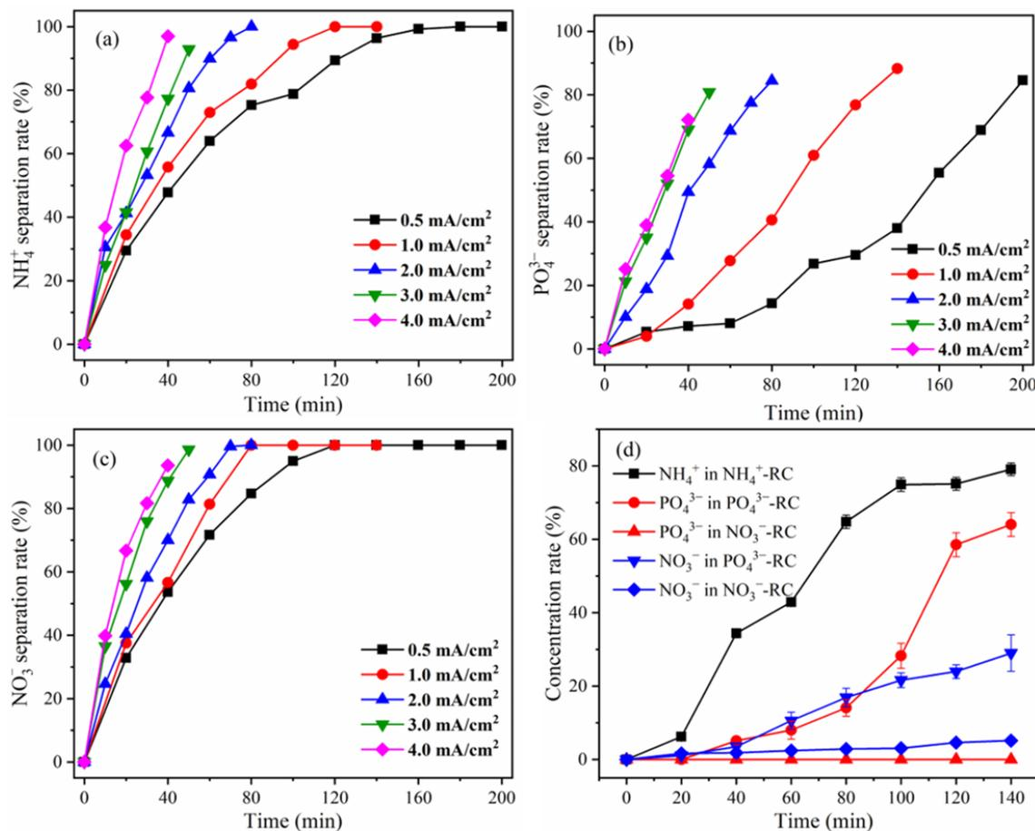
**Figure 3.** Effect of current density on the separation rate of (a)  $\text{NH}_4^+$ , (b)  $\text{PO}_4^{3-}$ , (c)  $\text{NO}_3^-$ , and (d) the concentration rate of  $\text{NH}_4^+$ ,  $\text{PO}_4^{3-}$ , and  $\text{NO}_3^-$  in different compartments under the condition of current density 1.0  $\text{mA/cm}^2$ .
