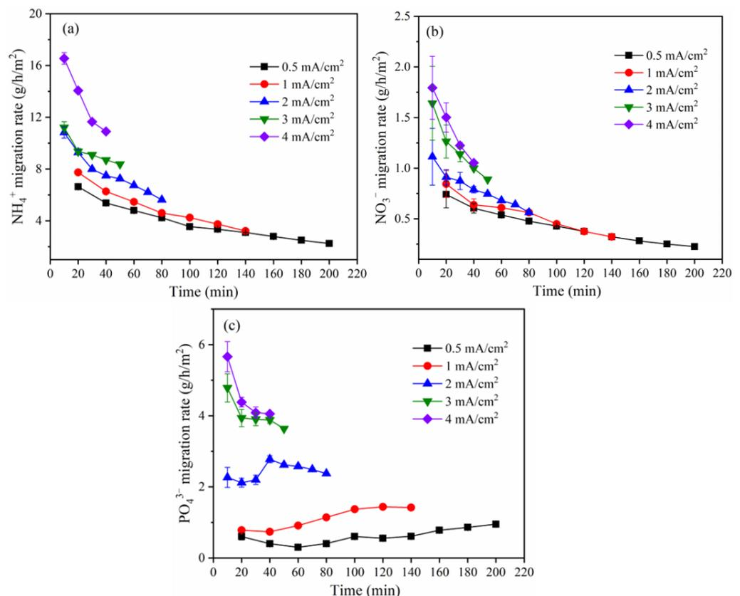
Figure 8. Migration rate of (a)  $\text{NH}_4^+$ , (b)  $\text{PO}_4^{3-}$ , and (c)  $\text{NO}_3^-$  under different current densities.
