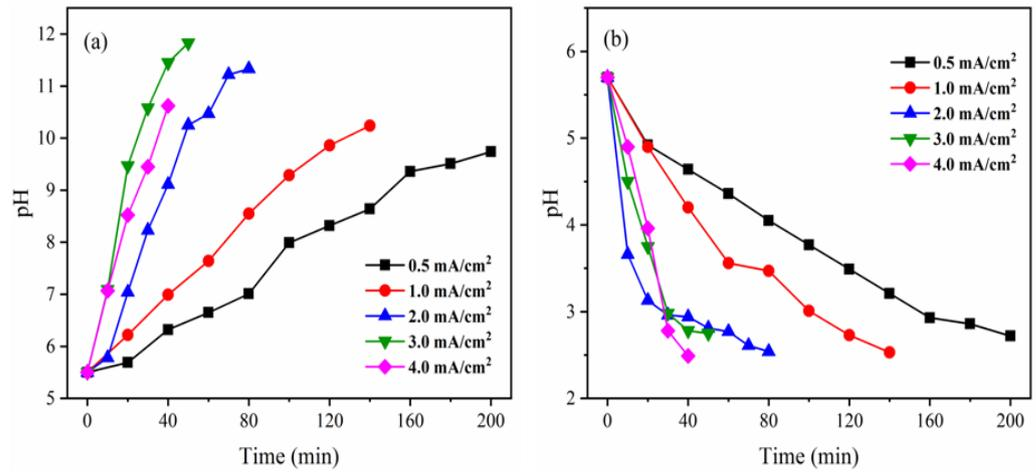
**Figure 5.** Effect of current density on (a) solution pH of ammonia compartment and (b) nitric acid compartment.
