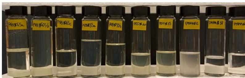
**Figure 7.** A representative picture of several PGEs considered in this study, from left to right are PVB#65a, PVB#65b, PVB#65c, PVB#55a, PVB#55b, PEO#10, PEO#15, PMMA#12, PMMA#18, PMMA#23 [65].
