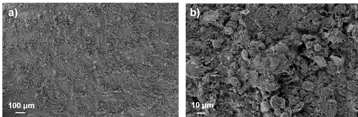
**Figure 2.** SEM images of the 5L anode microstructure obtained by printing ball-milled ink for three hours at 25 wt% of dry content (a)  $\times 150$  and (b)  $\times 1400$ .
