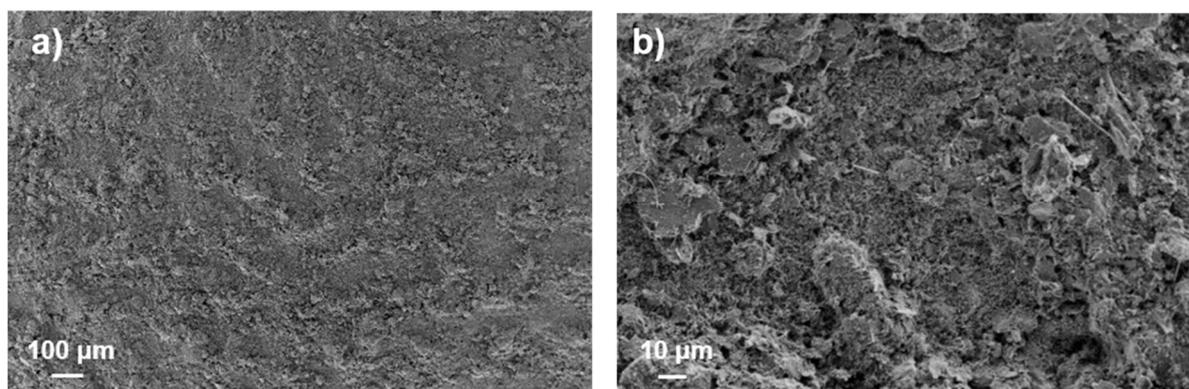
**Figure 4.** SEM images of the 6L anode microstructure obtained by printing ball-milled ink for three hours at 18 wt% of dry content using 90–10 % water–IPA solvent (a)  $\times 150$  and (b)  $\times 1400$ .
