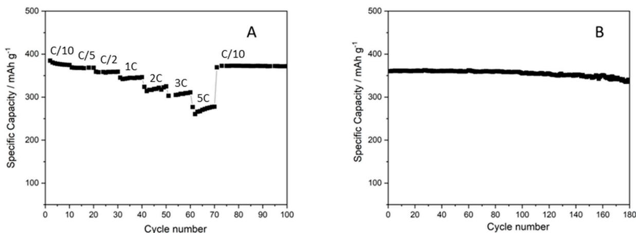
**Figure 5.** Discharge-specific capacity of the 6L anode microstructure obtained by printing ball-milled ink for three hours at 18 wt% of dry content using 90–10% water–IPA solvent at (A) variable and (B) C/10 constant rates.
