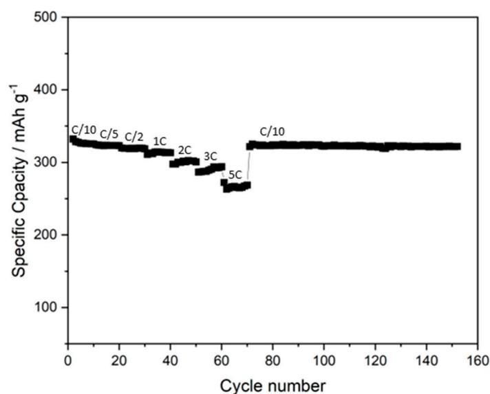
**Figure 3.** Discharge-specific capacity of the 5L anode obtained by printing ball-milled ink for three hours at 25 wt% of dry content at variable and constant rates.
