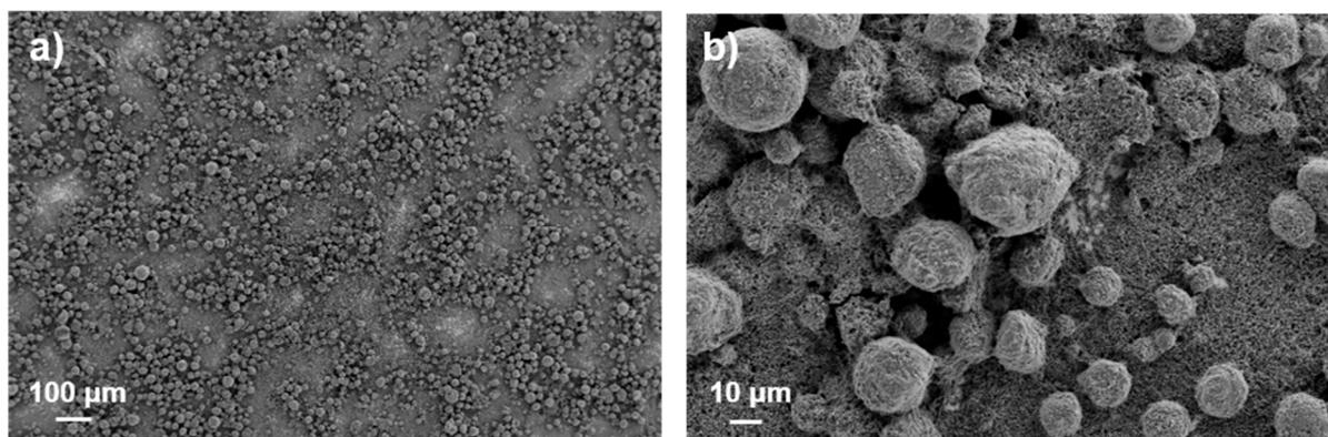
**Figure 1.** SEM images of the 5L anode microstructure obtained by printing ink at 25 wt% of dry content (a)  $\times 150$  and (b)  $\times 1400$ .
