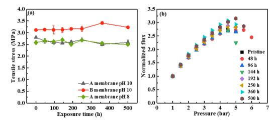
**Figure 4.** Changes in membrane mechanical properties with NaOCl exposure time. (**a**) Changes in the tensile stress of A and B membranes with NaOCl exposure time; and (**b**) changes in the collapse pressure of the C membrane with NaOCl exposure time.
