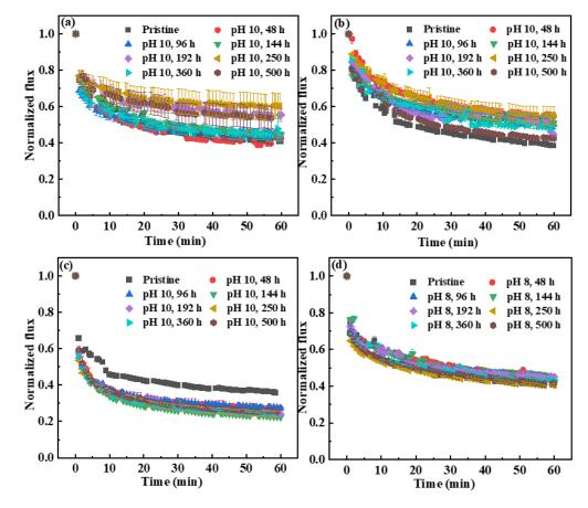
**Figure 6.** The fouling behaviors of the pristine and NaOCl-exposed membranes. (**a**) A membrane, NaOCl pH 10; (**b**) B membrane, NaOCl pH 10; (**c**) C membrane, NaOCl pH 10; and (**d**) A membrane, NaOCl pH 8.
