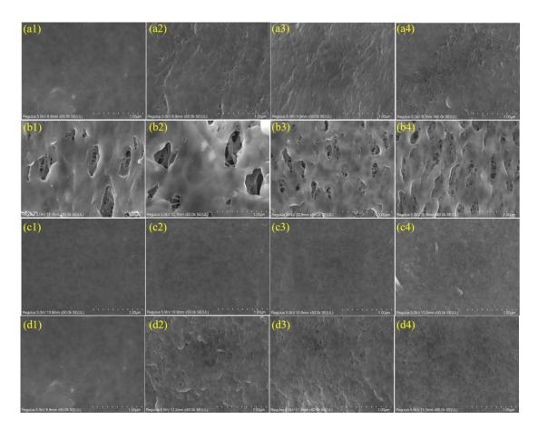
**Figure 1.** FESEM images of the outer surface morphologies of the pristine and NaOCl-exposed membranes. (**a1–a4**) A membrane, NaOCl Ph = 10; (**b1–b4**) B membrane, NaOCl pH = 10; (**c1–c4**) C membrane, NaOCl pH = 10; and (**d1–d4**) A membrane, NaOCl pH = 8; 1, 2, 3, and 4 represent exposure time 0, 48, 192, and 500 h, respectively.
