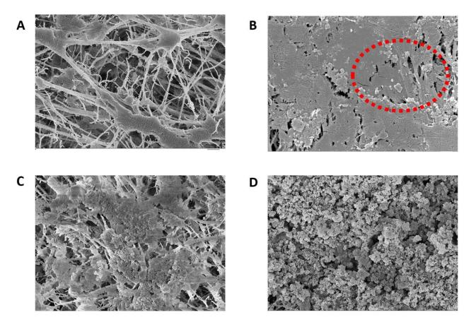
**Figure 8.** (A) SEM of pristine PTFE at 1  $\mu$ m, (B) SEM of seawater-fouled PTFE membrane at  $\mu$ m, the red circle indicates inorganic scaling, (C) SEM of landfill leachate wastewater-fouled PTFE membrane for 15 h at 1  $\mu$ m, and (D) SEM of membrane surface fouled with landfill leachate wastewater after 30 h of AGMD at 1  $\mu$ m.
