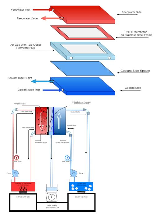
Figure 1. Schematic diagram of the AGMD unit.
