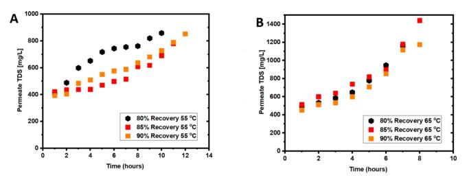
**Figure 3.** Permeate TDS for seawater treatment: (**A**) permeate TDS concentration for seawater treatment at 55 °C at 80%, 85%, and 90% recoveries; (**B**) permeate TDS concentration for seawater treatment at 65 °C at 80%, 85%, and 90% recoveries.
