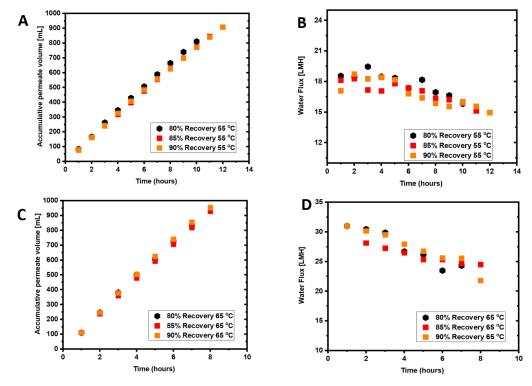
**Figure 2.** (**A**) Accumulative permeate volume at 55 °C, (**B**) water flux in the AGMD at 55 °C, (**C**) accumulative permeate volume at 65 °C, and (**D**) water flux at 65 °C. Feed solution: seawater (TDS = 32.8 g/L).
