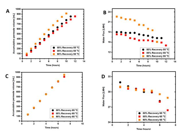
**Figure 5.** Permeate volume and water flux in AMGD: (**A**) 55 °C accumulative permeate volume; (**B**) 55 °C water flux in the AGMD; (**C**) 65 °C accumulative permeate volume, and (**D**) 65 °C water flux.
