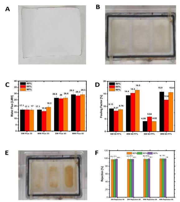
**Figure 10.** (**A**) Pristine membrane picture, (**B**) PTFE membrane after seawater treatment picture, (**C**) seawater average water flux with the fouling factors at 55 °C and 65 °C for all recoveries, (**D**) wastewater and seawater fouling factors at 55 °C and 65 °C for all recoveries, (**E**) picture of fouled wastewater membrane, and (**F**) comparison of seawater and wastewater rejection at 55 °C and 65 °C for all recovery rates.
