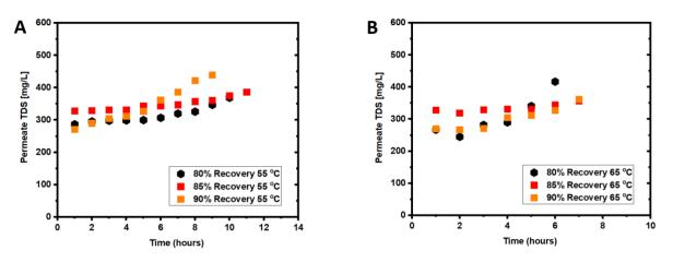
**Figure 6.** (**A**) Permeate TDS concentrations at 55 °C for 80%, 85%, and 90% recoveries; (**B**) permeate TDS concentrations at 65 °C for 80%, 85%, and 90% recoveries.
