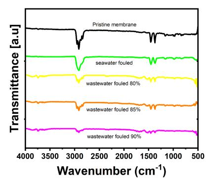
**Figure 9.** FT-IR bands of pristine and fouled membranes by seawater and wastewater at different recoveries.
