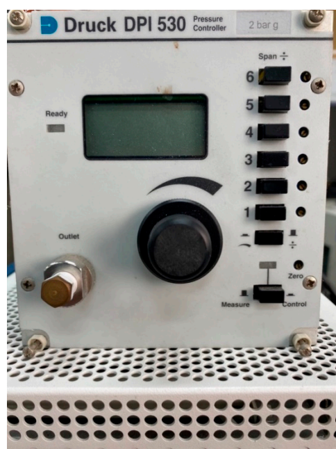
Figure 8. A Druck-DPI 530 pressure controller.
