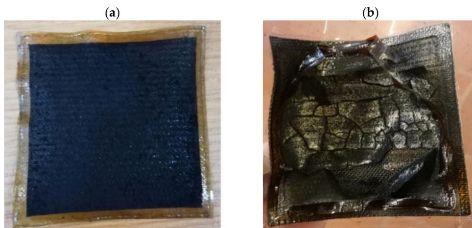
**Figure 16.** Digital images of polybenzimidazole (PBI) membranes before and after ammonia exposure: (a) fresh membrane (before) and (b) cracked membrane (after).
