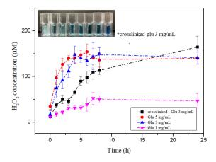
**Figure 5.** Effect of glucose concentration loaded in Glu/PVA dope and GA crosslinking on the time course of  $H_2O_2$  generation from the GOx/Glu membranes.
