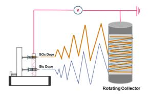
Figure 1. Simultaneous electrospinning of GOx/PVA and Glu/PVA interwoven nanofibrous membrane.
