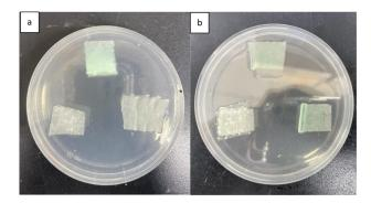
**Figure 4.** Qualitative test of H2O2 generation from pristine membranes; (**top**) co-electrospun GOx/Glu/PVA; (**bottom left**) PVA only; (**bottom right**) PVA/Gox. DA-64 and HRP colorimetric assay employed for producing Bindschedler's green on agar plate (**a**) without; (**b**) with 0.8% glucose supplement in the agar.
