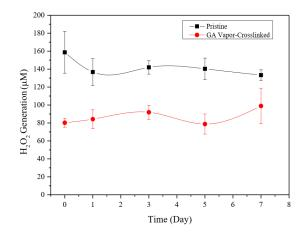
**Figure 6.** Stability GOx encapsulated in PVA nanofibrous membrane (with and without vaporcrosslinking) with Glu 3 mg/mL in Glu/PVA dope as measured by its hydrogen peroxide generation capacity at 4 h reaction time after being kept at room temperature for different days.
