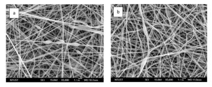
**Figure 2.** FE-SEM micrographs of simultaneously co-electrospun PVA/GOx-PVA/Glu nanofibrous membrane; (**a**) before GA vapor crosslinking; (**b**) after GA vapor crosslinking.
