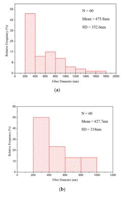
**Figure 3.** Diameter size distribution of nanofibers consisted of the simultaneous electrospun nanofibrous membrane; (**a**) before GA vapor-crosslinking; (**b**) after GA vapor-crosslinking.
