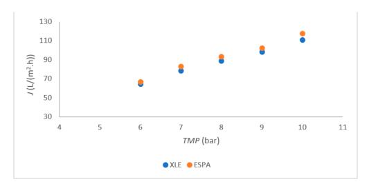
**Figure 2.** Flux in dependence of *TMP* for both membranes.
