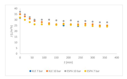
Figure 3. Flux dependent on time for both membranes.
