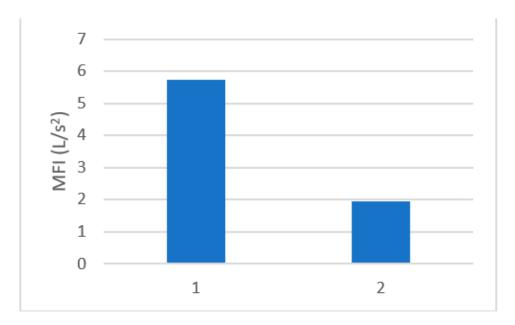
Figure 5. MFI for 1. Untreated mixed wastewater, 2. Pre-treated mixed wastewater.
