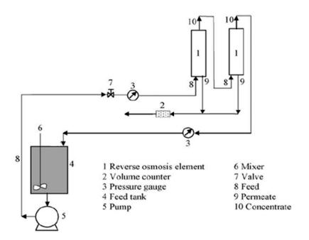
Figure 1. Schematic RO process.
