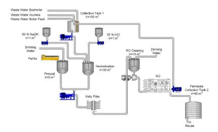
Figure 7. Schematic process scheme for wastewater treatment.
