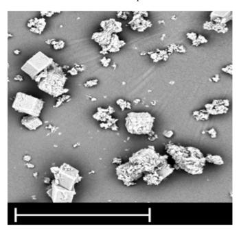
Figure 6. SEM image of deposit from the membrane after cleaning (line: 10 μm).
