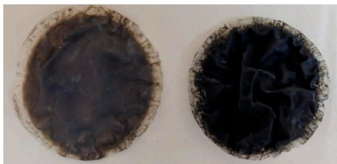
**Figure 8.** 2% rGO/TiO<sub>2</sub> membrane before (left) and after 96 h of use (right).
