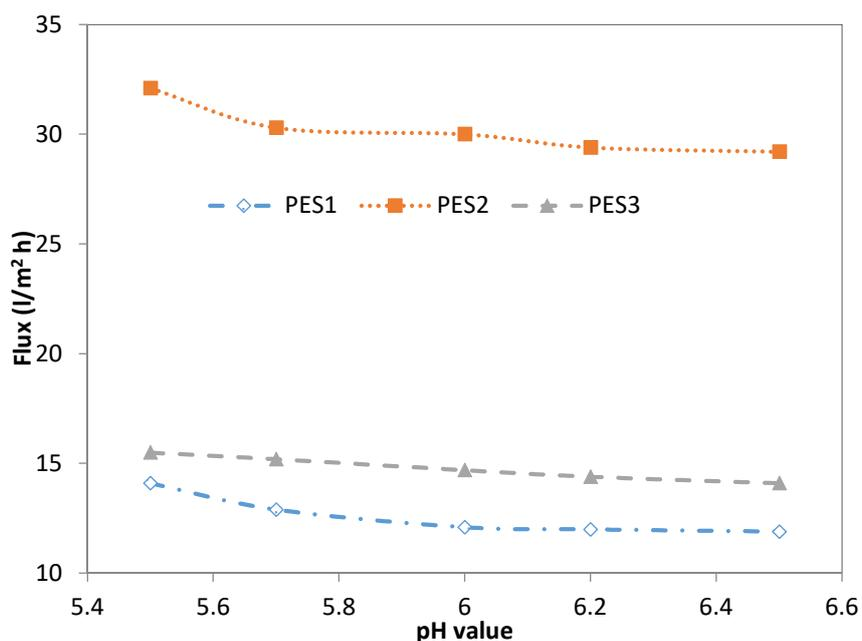
**Figure 3.** Effect of feed pH value on final permeate flux of PES1, PES2, and PES3 membranes for Pb<sup>2+</sup> (experimental conditions: Pb<sup>2+</sup> concentration of 100 ppm, transmembrane pressure of 1 bar).
