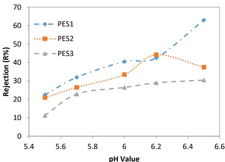
**Figure 6.** Effect of feed pH on  $Cd^{2+}$  rejection of PES1, PES2, and PES3 membranes (experimental conditions:  $Cd^{2+}$  concentration of 100 ppm, and transmembrane pressure of 1 bar).
