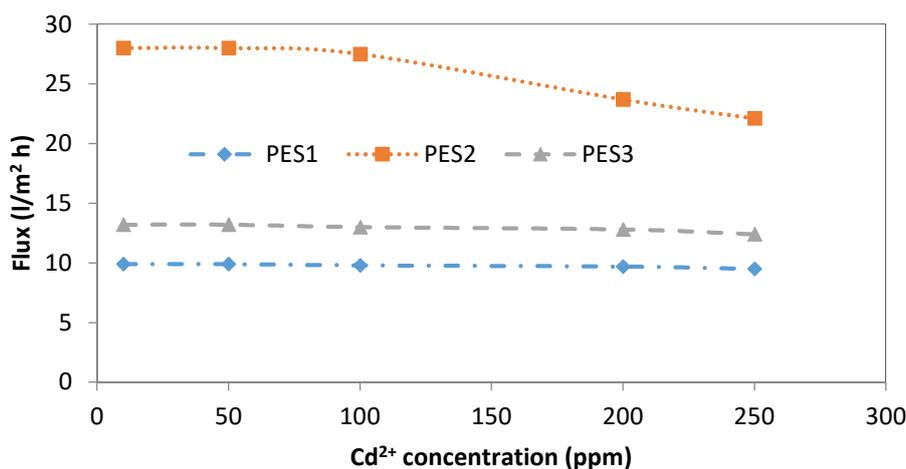
**Figure 8.** Effect of Cd<sup>2+</sup> initial concentration on permeate flux of PES1, PES2, and PES3 membranes (experimental conditions: pH = 6 ± 0.2, transmembrane pressure of 1 bar).
