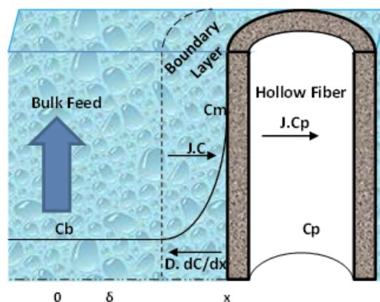
Figure 2. Schematic diagram of concentration polarization phenomenon in hollow fiber.
