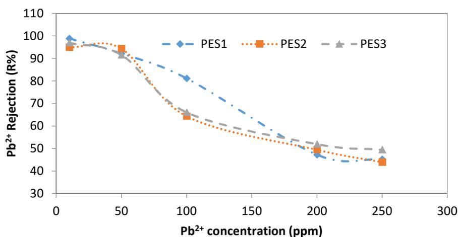
**Figure 9.** Effect of initial Pb<sup>2+</sup> concentration on Pb<sup>2+</sup> rejection using PES1, PES2, and PES3 membranes (experimental conditions: pH = 6 ± 0.2, transmembrane pressure of 1 bar).
