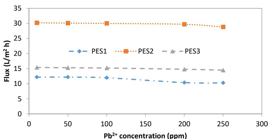
**Figure 7.** Effect of Pb<sup>2+</sup> initial concentration on permeate flux of PES1, PES2, and PES3 membranes (experimental conditions: pH = 6 ± 0.2, transmembrane pressure of 1 bar).
