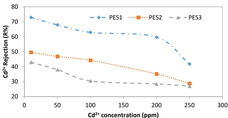
**Figure 10.** Effect of initial Cd<sup>2+</sup> concentration on Cd<sup>2+</sup> rejection using PES1, PES2, and PES3 membranes (experimental conditions: pH = 6 ± 0.2, transmembrane pressure of 1 bar).
