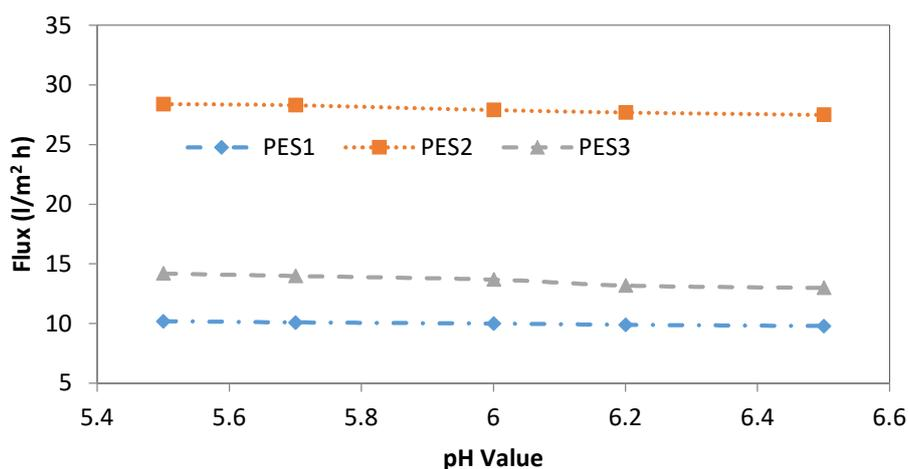
**Figure 4.** Effect of feed pH value on final permeate flux of PES1, PES2, and PES3 membranes, (experimental conditions: Cd<sup>2+</sup> concentration of 100 ppm, transmembrane pressure of 1 bar).
