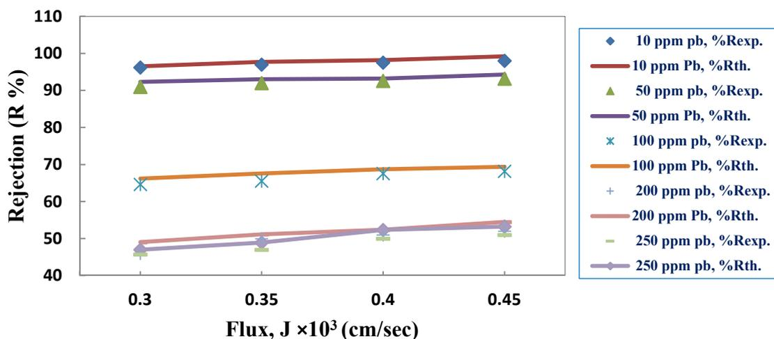
Figure 11. Results of CFSK model for the dataset of the PES3 membrane for Pb(NO<sub>3</sub>)<sub>2</sub>.
