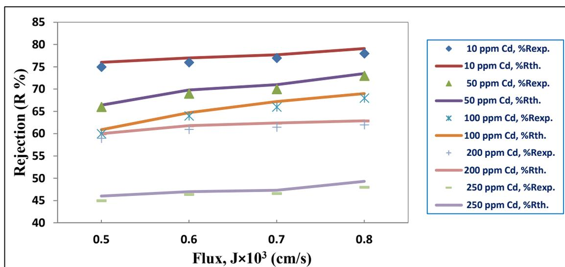
Figure 12. Results of CFFP model for the dataset of the PES1 membrane for Cd(NO<sub>3</sub>)<sub>2</sub>.
