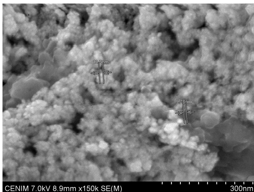
Figure 7. SEM image of the precipitated gold nanoparticles. Marked particles size: 13.2 nm (upper), 9.28 nm (lower).
