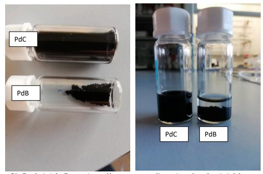
**Figure S3.** Catalytic ink. Comparison of homogeneous dispersion of catalyst in ink between PdC and PdB. The suspensions were sonicated in exaggerated time (2 h) to be able to appreciate the aggregation of particles of unsupported catalyst with naked eye.
