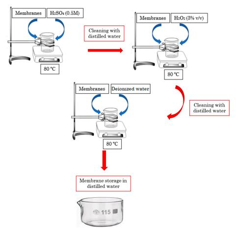
Figure S1. Nafion membrane cleaning procedure:
