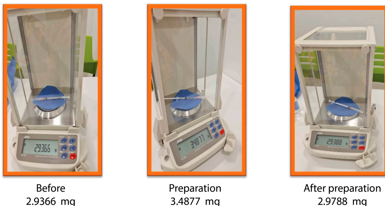
Figure 3. Comparison of vaccine weights by using the air-filled technique. Before: Weight of the empty syringe and needle. Preparation: Filled syringe with the vaccine. After preparation: Weights of the syringe and needle after injection.
