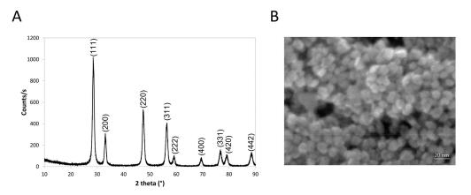
**Figure 1.** Nanoceria physicochemical characterization. **(A)** XRD diffraction patterns and Miller indexes of nanoceria. **(B)** Scanning electron microscopy (SEM) image of nanoceria. The scale bar corresponds to 20 nm.
