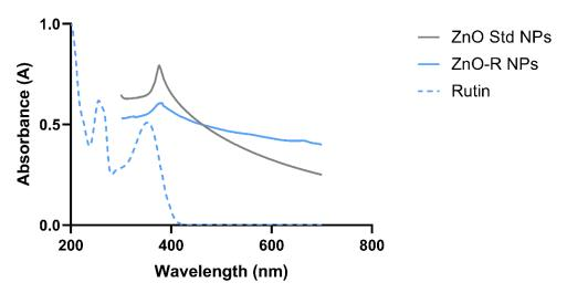
Figure 5. UV-Vis absorption spectra of ZnO Std NPs, ZnO-R NPs and rutin.
