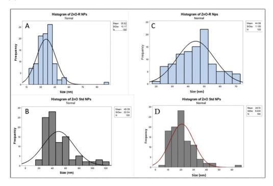
**Figure 2.** Histogram from the SEM of (**A**) ZnO-R NPs and (**B**) ZnO Std NPs. Histogram from the TEM of (**C**) ZnO-R NPs and (**D**) ZnO Std NPs.
