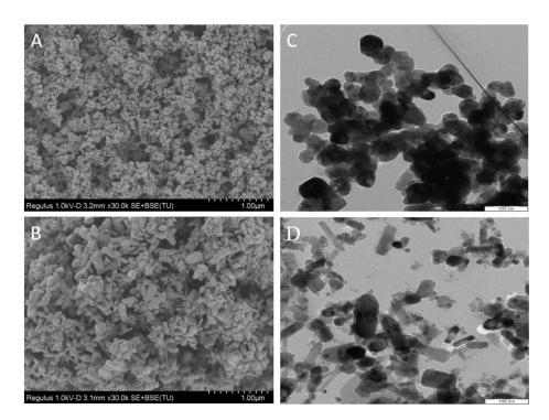
**Figure 1.** SEM images of (**A**) ZnO-R NPs and (**B**) ZnO Std NPs. TEM images of (**C**) ZnO-R NPs and (**D**) ZnO Std NPs.
