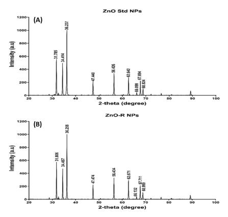
Figure 4. XRD of (A) ZnO Std NPs and (B) ZnO-R NPs.
