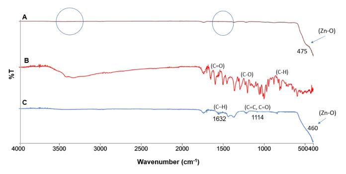
Figure 3. ATR-FTIR spectra of (A) ZnO Std NPs, (B) rutin and (C) ZnO-R NPs.
