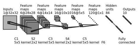
Figure 3. The architecture of LeNet-5.
