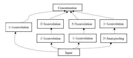
Figure 4. The architecture of the Inception V1 module.
