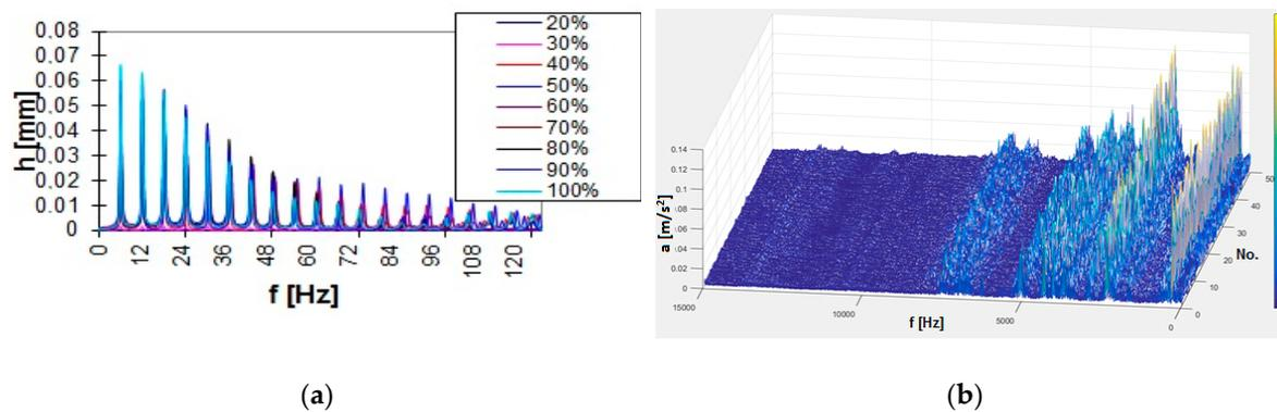
**Figure 5.** Influence of the fuel setting in the range of 20–100% on the spectrum of displacement vibration signals in the 0–125 Hz frequency band (a); the cascade spectrum of the vibration acceleration signal in the injection subsystem in the 0–15 kHz frequency band (b):  $f$ —frequency.
