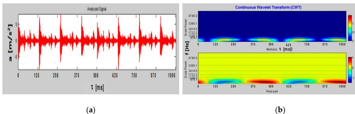
**Figure 7.** An example of original acceleration vibration signal (a) and continuous wavelet transform (b).
