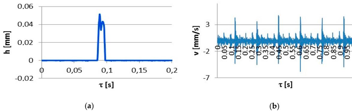
**Figure 4.** Sample time waveforms of the displacement vibration signal  $h$  of the injector needle for the fuel setting 70% (a); time waveforms of the vibration velocity signal  $v$  processed in the injection subsystem in the frequency range 0–20 kHz at a 40% relative load of engine (b):  $\tau$ —time.
