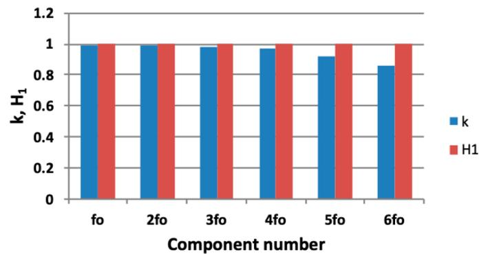
**Figure 8.** Correlation coefficient  $k$  and results of  $H_1$  alternative hypothesis testing (1), that the input quantities (dose of fuel) in preliminary studies are correlated for the symptoms of spectral vibration displacements;  $f_o$ —rotational frequency.
