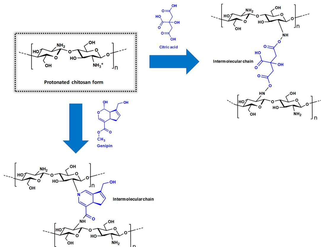
Figure 5. The mains cross-linking reactions using chitosan.
