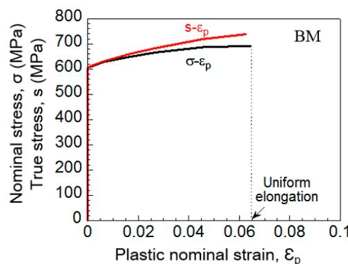
Figure 5. Stress-strain curves for HSB600 steel.
