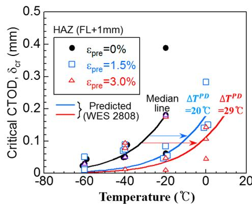
**Figure 8.** Temperature shift  $\Delta T_{PD}$  for the pre-strained HAZ predicted with the procedure specified in WES 2808.
