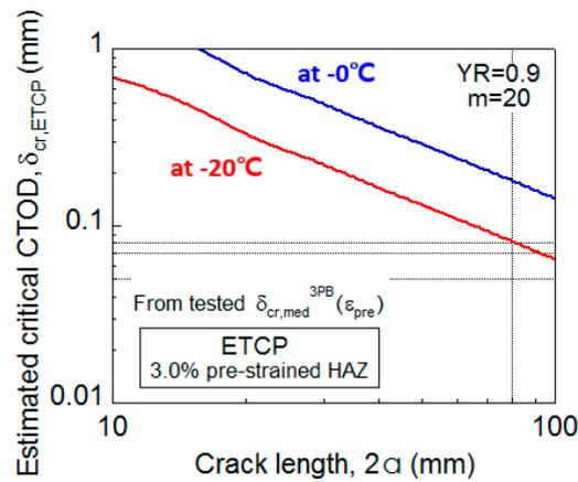
Figure 6. Critical CTODs for the 3.0% pre-strained ETCP estimated from 3.0% pre-strained (three-point bend) 3PB test results.
