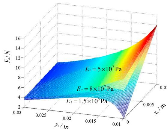
**Figure 11.** Influences of  $x_o$ ,  $y_o$ , and  $E$  on  $F_o$  ( $r = 0.02$  m,  $R_o = 0.01$  m,  $l = 0.03$  m,  $r_p = 0.003$  m,  $N = 12$ ,  $p_o = 1.01 \times 10^5$  Pa, and  $p_i = 0.8 p_o$ ).
