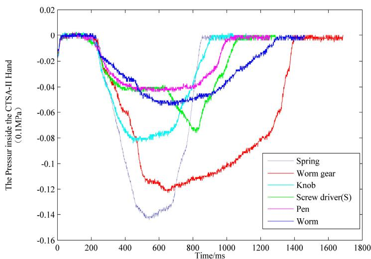
**Figure 20.** The change of internal pressure when the CTSA-II hand grasps objects.
