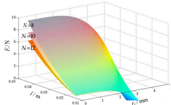
**Figure 10.** Influences of  $r_p$ ,  $l$ , and  $N$  on  $F_o$  ( $r = 0.02$  m,  $R_o = 0.015$  m,  $x_o = 0$ ,  $y_o = 0.03$  m,  $E = 5 \times 10^7$  Pa,  $p_o = 1.01 \times 10^5$  Pa, and  $p_i = 0.8 p_o$ ).
