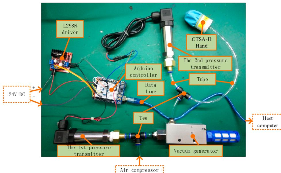
**Figure 17.** The experimental platform of exploring pressure.
