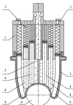
**Figure 5.** The expected improved design of CTSA hand, including components: 1, base; 2, spring; 3, balloon membrane; 4, pins; 5, gas or fluid; 6, object.
