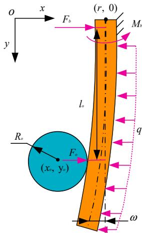
**Figure 9.** Force analysis of single pin.
