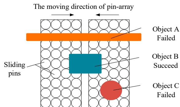
**Figure 2.** The objects that omnigripper can or cannot crawl.
