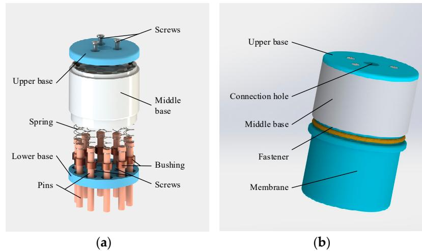
**Figure 6.** The design of the CTSA-II hand: (a) the explosion view, (b) the overall appearance.
