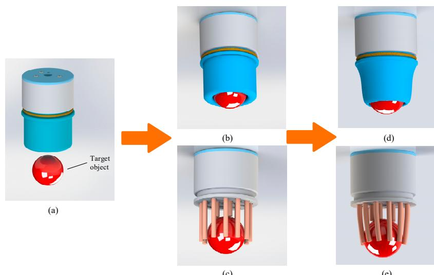
**Figure 7.** Grasping process of the robot hand: (a) before grasping, (b) self-adaptive step, (c) self-adaptive step hiding membrane, (d) gripping step, and (e) gripping step hiding membrane.
