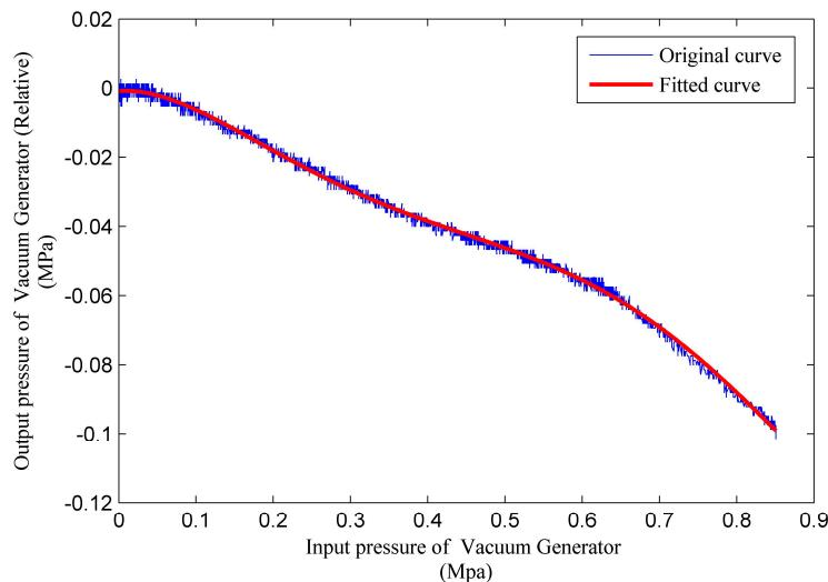
**Figure 19.** The characteristics of the vacuum generator used in the system of CTSA-II hand.
