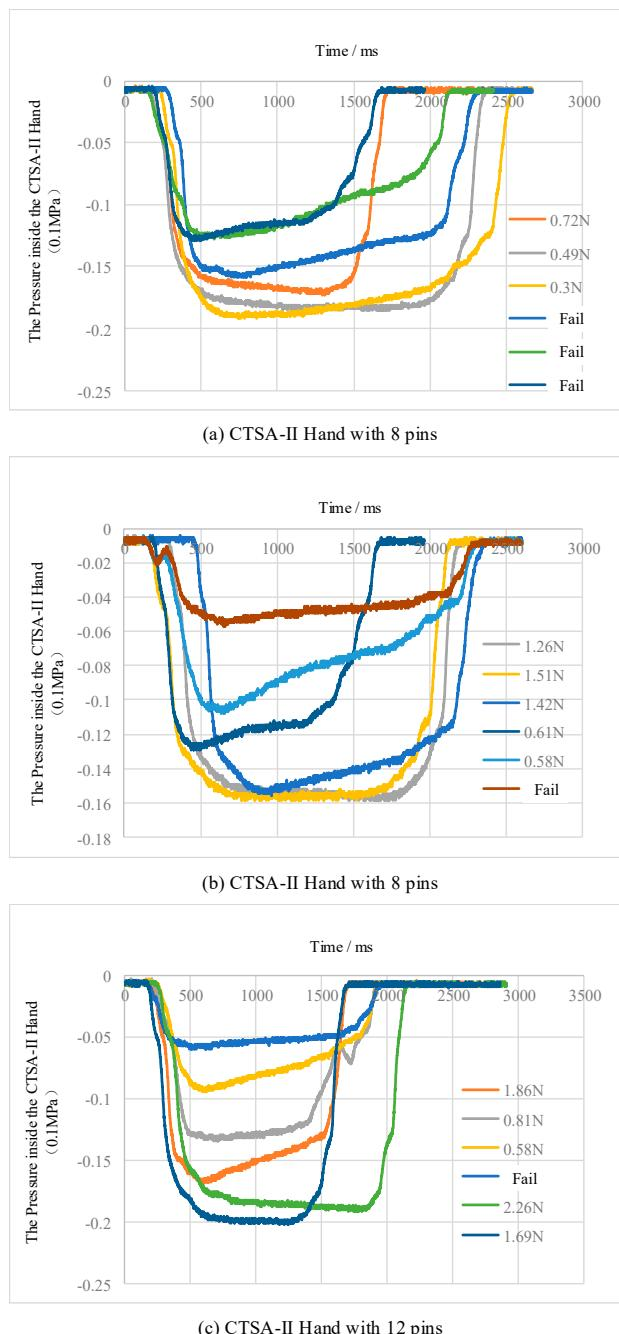
**Figure 22.** The relationships between the internal pressure and the grasping force.
