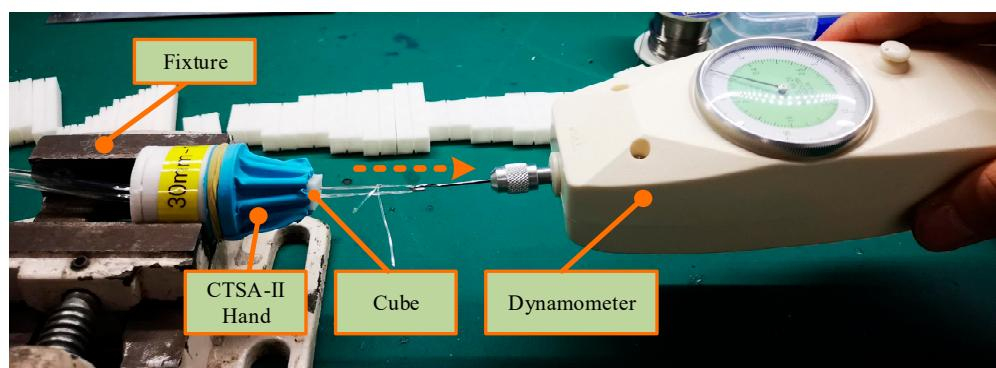
**Figure 21.** The experiment of measuring the grasping force.
