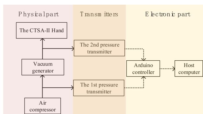
**Figure 18.** The experimental structure of exploring pressure.
