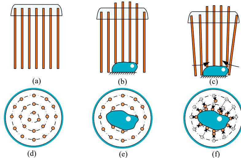
**Figure 3.** The cluster tube self-adaptive (CTSA) grasping mode.
