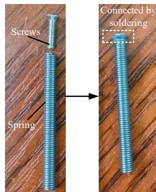
**Figure 13.** The composition of the pin.
