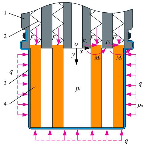
**Figure 8.** The overall force situation: 1, base; 2, spring; 3, balloon membrane; 4, bendable sliding pins.
