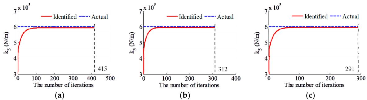
**Figure 7.** Comparison of the identified  $k_5$  using different numbers of sample points: (a) using 300 sample points; (b) using 600 sample points; (c) using 900 sample points.
