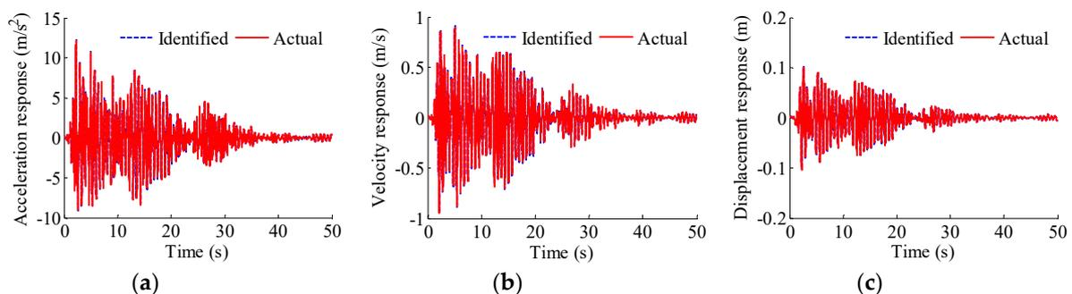
**Figure 6.** Comparison of the structural responses on the top floor (10% noise): (a) acceleration; (b) velocity; (c) displacement.
