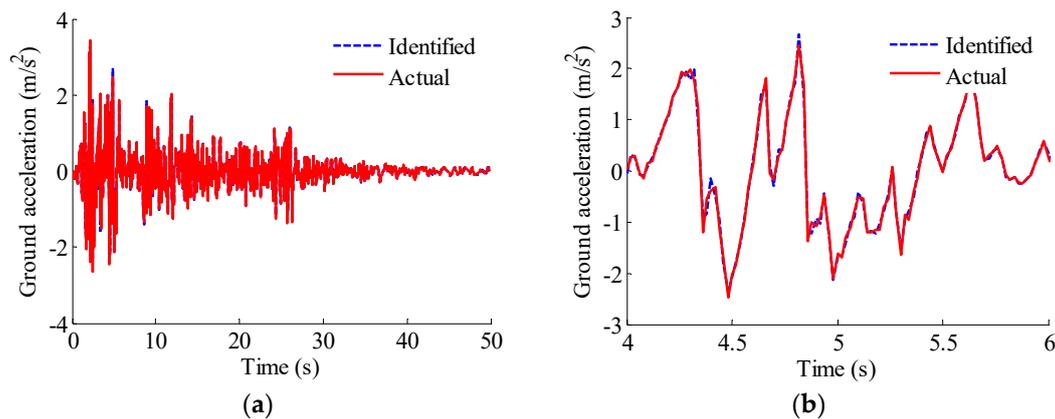
**Figure 5.** Identified results of the ground acceleration (10% noise): (a) the whole time history; (b) the time segment from 4 s to 6 s.
