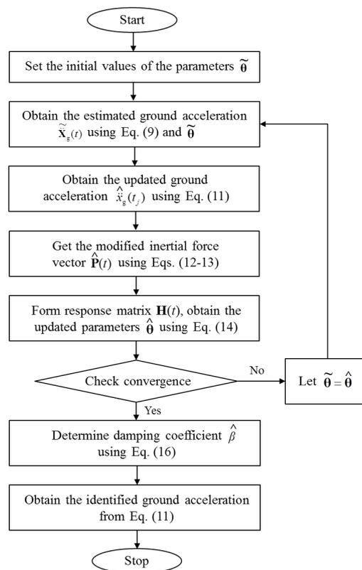
Figure 1. Flowchart of the proposed iterative identification procedure.
