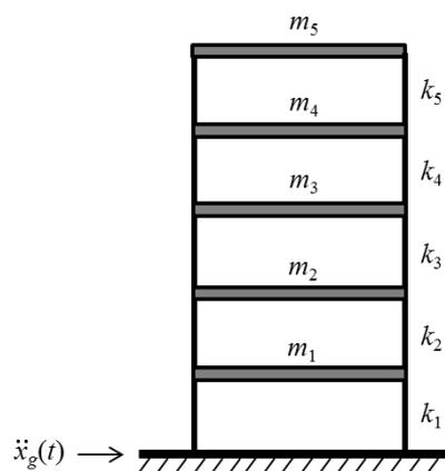
Figure 2. Five-story building model in the numerical example.
