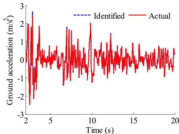
Figure 10. Identified results of the ground acceleration (15 times).
