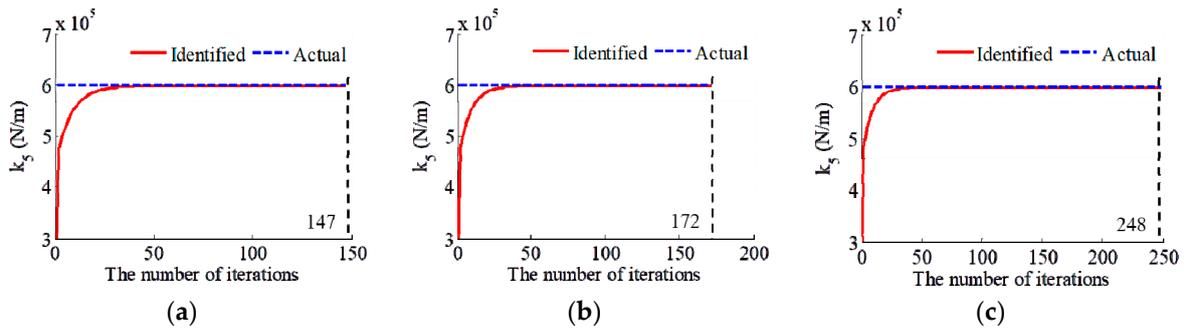
**Figure 3.** Comparison of the effect of noise intensity on the iteration process: (a) noise-free; (b) 5% noise; (c) 10% noise.
