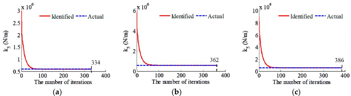
Figure 9. Comparison of the identified  $k_5$  with different initial values: (a) 5 times; (b) 10 times; (c) 15 times.
