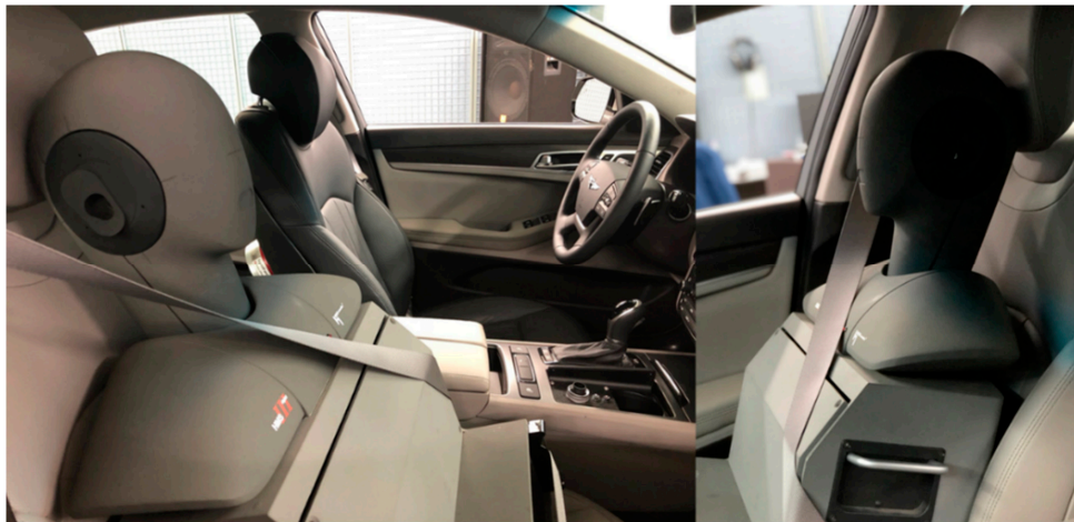
Figure 2. Dummy head used in the study and an example of the installation.
