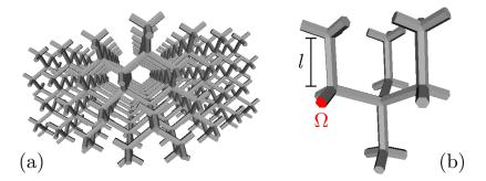
**Figure 1.** (a) Diamond lattice made of interconnected rods. A small part of the structure is detailed in (b).
