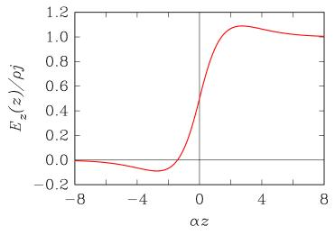
**Figure 4.** Variation of the electric field predicted by Equation (21) in the effective medium representing a 3D conductive mesh. The upper half space z > 0 is crossed by a uniform current of density *j* flowing in the *z* direction. There is no current in the lower half space z < 0.
