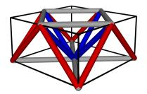
**Figure 2.** Half the conventional unit cell (thin black lines) of a face-centered cubic resistor lattice. The resistive rods represented in gray interconnect nodes located within the same horizontal plane. The blue rods are located inside the unit cell. The red rods, located in the vertical faces, are shared by two adjacent cubic cells.
