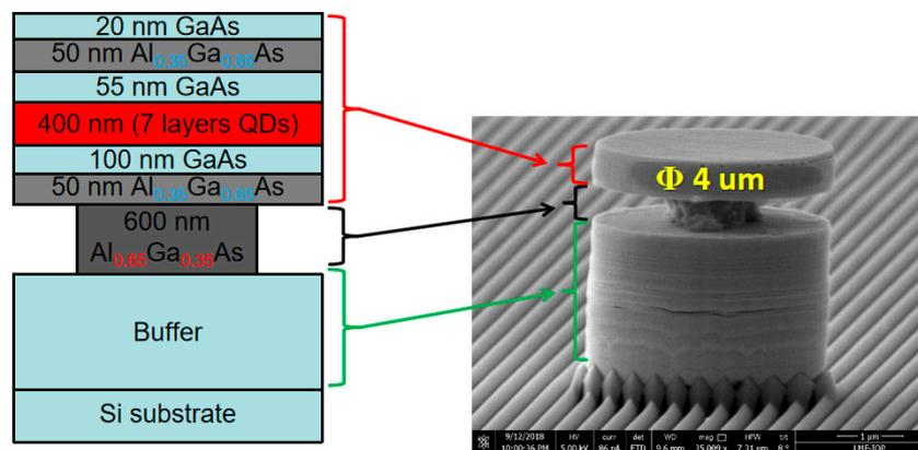
Figure 8. Schematic diagram and SEM image of InAs QD microdisk laser structure.
