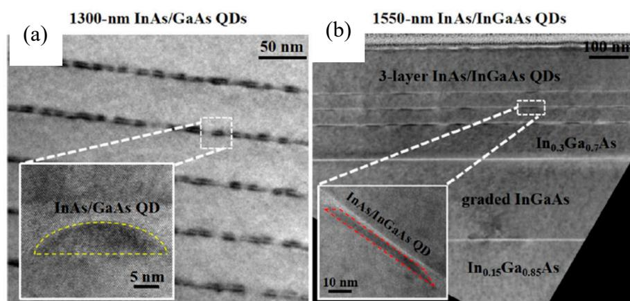
**Figure 3.** (a) Cross-sectional TEM image of a five-layer InAs QDs grown on the sawtooth hollow structured Si (001) substrate for O-band emission. Inset: High resolution TEM image of an InAs/GaAs QD. (b) Cross-sectional TEM image of three-layer InAs QDs on the InGaAs/GaAs/Si (001) substrate for C/L-band emission. Inset: High resolution TEM image of a trapezoidal InAs/InGaAs QD.
