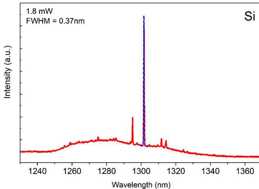
**Figure 10.** Laser spectrum for a 4  $\mu\text{m}$  InAs/GaAs QD microdisk laser on Si.
