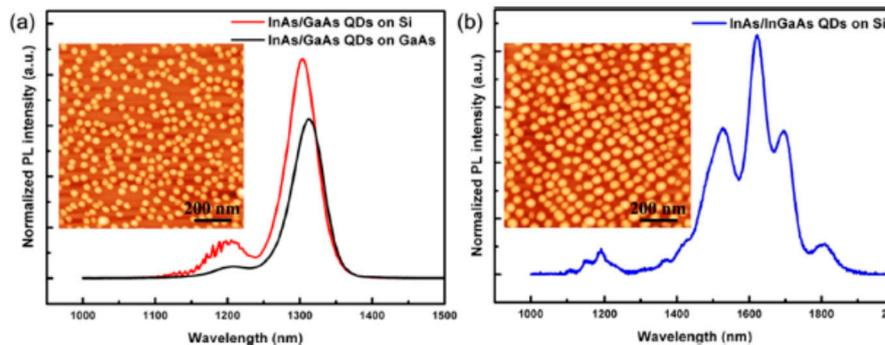
**Figure 5.** Room temperature photoluminescence spectra of (a) InAs/GaAs QDs grown on GaAs and Si (001) substrates for O-band emission and (b) InAs/InGaAs QDs grown on Si (001) substrates for C/L-band emission. Insets:  $1\ \mu\text{m} \times 1\ \mu\text{m}$  AFM image of (a) InAs/GaAs QDs on Si and (b) InAs/InGaAs QDs on Si.
