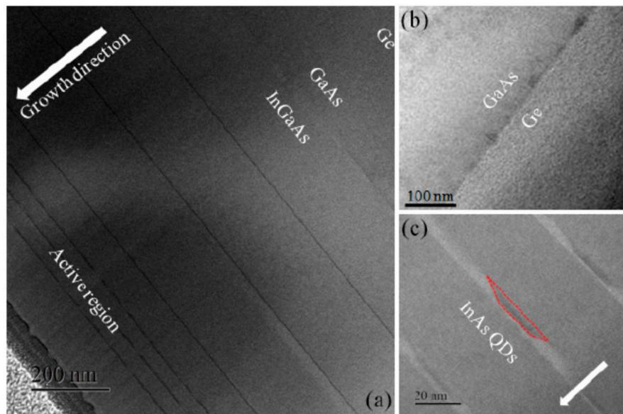
**Figure 1.** (a) The STEM image of C/L-band InAs quantum dots structure on Ge substrate. The white arrow: The growth direction of the epitaxial layers. (b) Bright field TEM image of GaAs/Ge interface. (c) High magnification STEM image of InAs QDs. The red-marked region: The cross section of a top-flattened InAs QD. All images are taken along [110] direction.
