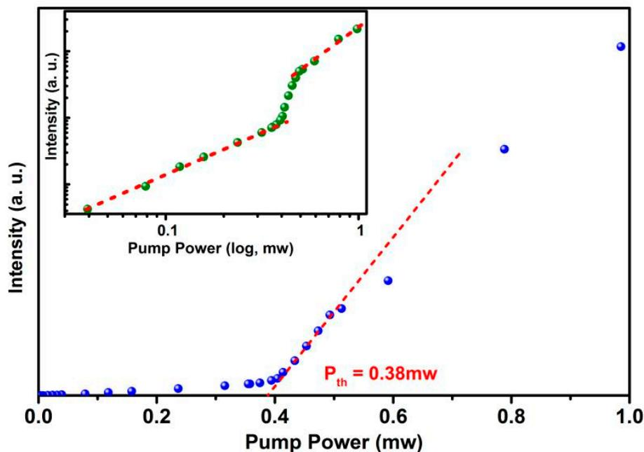
Figure 9. L-L curve of InAs/GaAs QD microdisk laser grown on (111)-faceted hollow Si (001) substrate; inset: double log plot of the S-curve.
