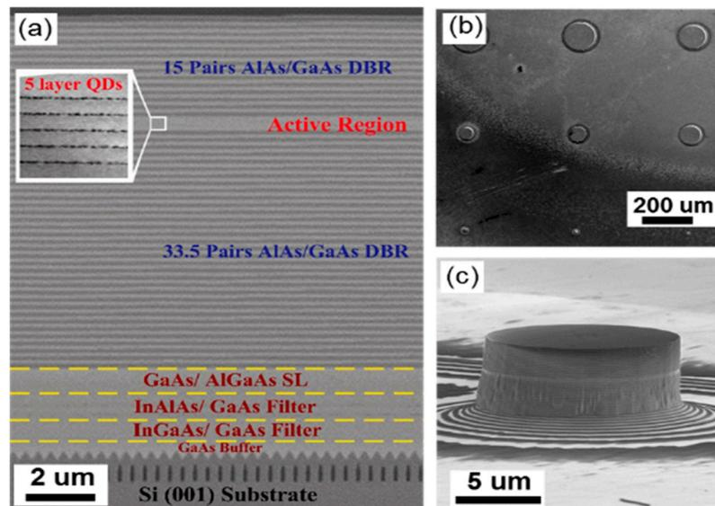
**Figure 6.** (a) The cross-sectional SEM image of InAs/GaAs micropillar laser structure on (111)-faceted Si (001) hollow substrate; InAs/GaAs QDs embedded in one  $\lambda$ -cavity with 15 (33.5) pairs of top (bottom) DBRs; (b) top-view SEM image of micropillar lasers with different diameters; (c) tilted SEM image of InAs/GaAs QD micropillar laser on Si (001) with 15  $\mu\text{m}$  diameter.
