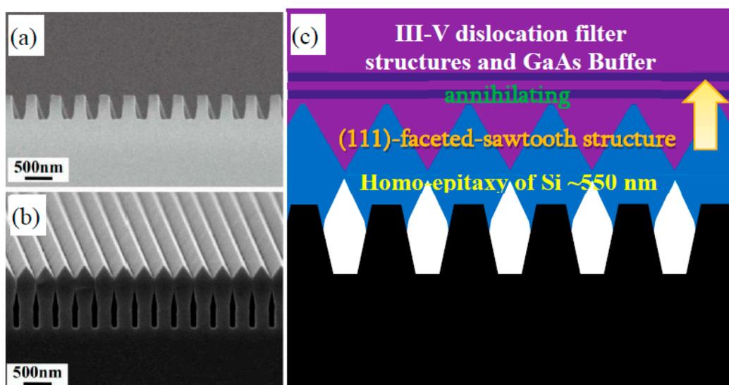
**Figure 2.** (a) Cross-sectional scanning electron microscope image of U-shape Si (001) substrate, (b) (111)-faceted-sawtooth structure epitaxial growth on U-shape Si (001) hollow substrate, and (c) schematic diagram of epitaxial growth of (111)-faceted hollow structure on U-shape Si (001) substrate.
