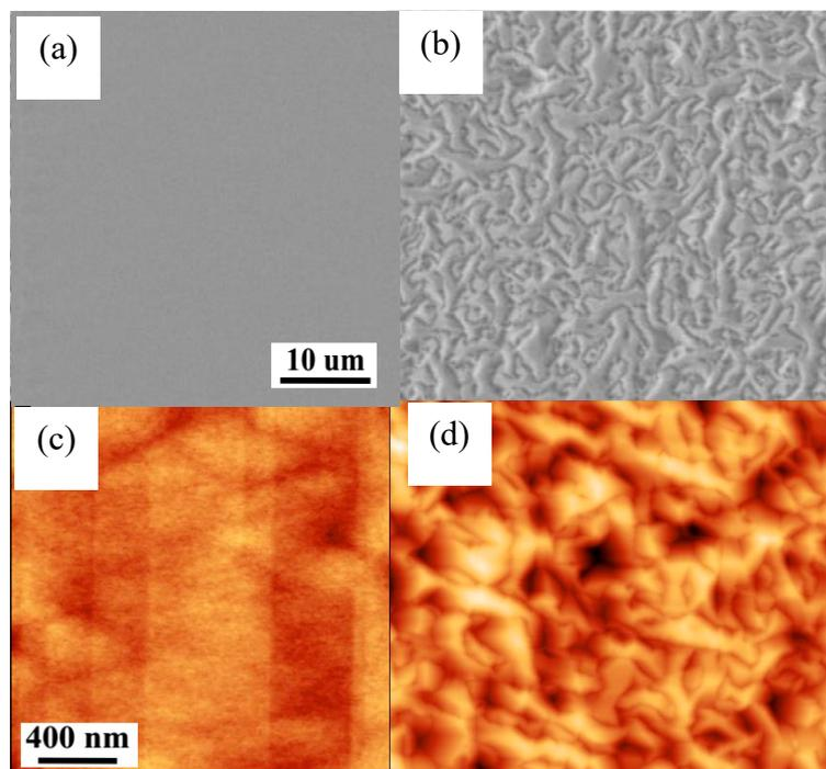
**Figure 4.** Top-view SEM images of GaAs grown on (a) (111)-faceted sawtooth-structured Si (001) and (b) standard Si (001) substrates, and  $2\ \mu\text{m} \times 2\ \mu\text{m}$  atomic force microscope (AFM) images of GaAs film on (c) (111)-faceted Si (001) hollow structure and (d) GaAs/Si substrate.
