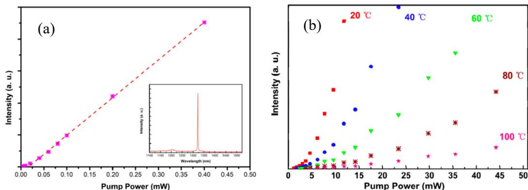
**Figure 7.** (a) Output intensity as a function of pump power (L-L curve) of InAs/GaAs QD micropillar laser on Si at room temperature. Inset: spectral plot of micropillar laser at the pump power of 6 mW. (b) Integrated PL intensity of InAs QD micropillar on Si (001) as a function of pump power of temperature ranging from 20 to 100  $^{\circ}\text{C}$ .
