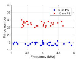
**Figure 9.** Fringe number trend with SMI signal Doppler frequency of PS particles in different diameters. The blue circles denote  $5 \mu m$  and the red squares denote  $10 \mu m$ .
