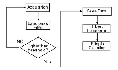
Figure 6. Flow chart drawing of the data acquisition and processing algorithm.
