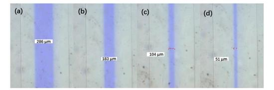
**Figure 7.** Photographs of the dye fluid in the focusing chamber with sheath-sample-sheath flow rate: (a) 15 μL/min–20 μL/min–15 μL/min; (b) 20 μL/min–10 μL/min–20 μL/min; (c) 20 μL/min–5 μL/min–20 μL/min; (d) 32 μL/min–4 μL/min–32 μL/min.
