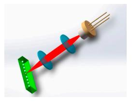
**Figure 4.** Schematic experimental setup. The system consists of a laser diode, doublet lenses optical arrangement, and microchannel.
