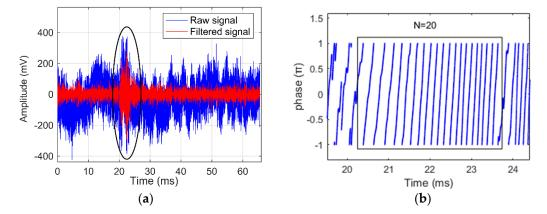
**Figure 8.** Data processing on the SMI signal from a polystyrene sphere particle of 8 μm diameter. (**a**) Raw SMI signal (blue) and filtered SMI signal by a home-made band-pass filter (red). (**b**) Instantaneous phase visualization via Hilbert transform to interfere with fringe number retrieving (in the frame).
