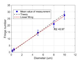
**Figure 11.** The fringe number of the SMI signal burst as a function of particle diameter. The error bars represent the standard deviation values. The black dashed line denotes the calculation result from Equation (7).
