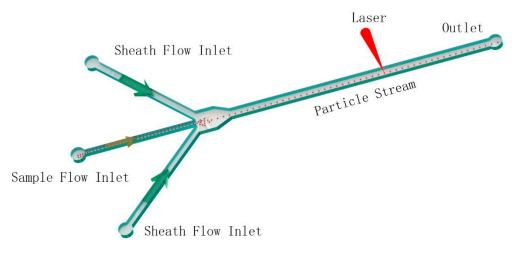
Figure 5. Schematic of the hydrodynamic focusing channel.
