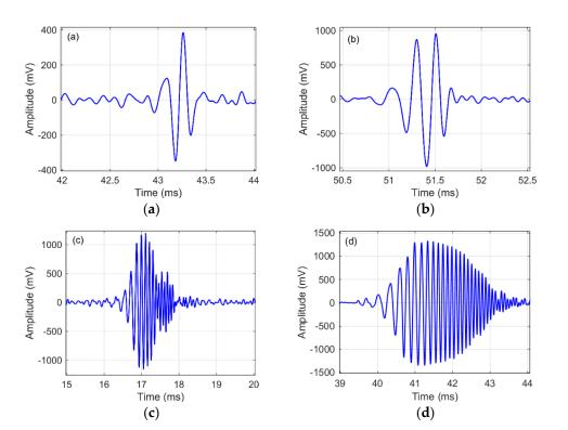
**Figure 10.** Signal burst of the PS particle in different diameters: (**a**) 200 nm; (**b**) 500 nm; (**c**) 5  $\mu$ m; (**d**) 10  $\mu$ m.
