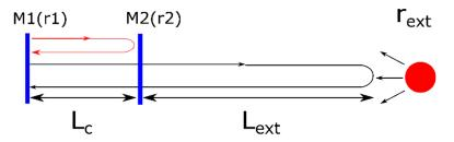
Figure 1. Schematic three-mirror cavity model.
