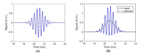
**Figure 3.** Simulated self-mixing interferometry (SMI) signal in the presence of an individual flowing particle. (**a**) The Gaussian-shaped sinusoidal SMI signal. (**b**) The synthesized SMI signal consisting of sinusoidal signal oscillation and pedestal.
