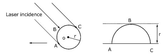
**Figure 2.** Laser incidence process upon the flowing particle and external cavity length variation  $\Delta L$  from point A to C.
